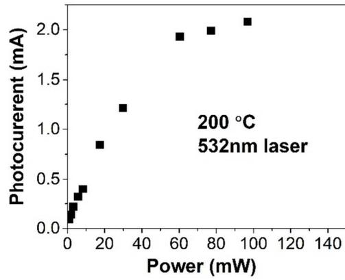
Figure S1: Photocurrents of detector based on RGO thin film prepared by eight cycles of drop-casting and annealing at 200 °C as a function of illumination power under laser illumination of 532 nm (VIS) at a bias voltage of 0.5 V.
