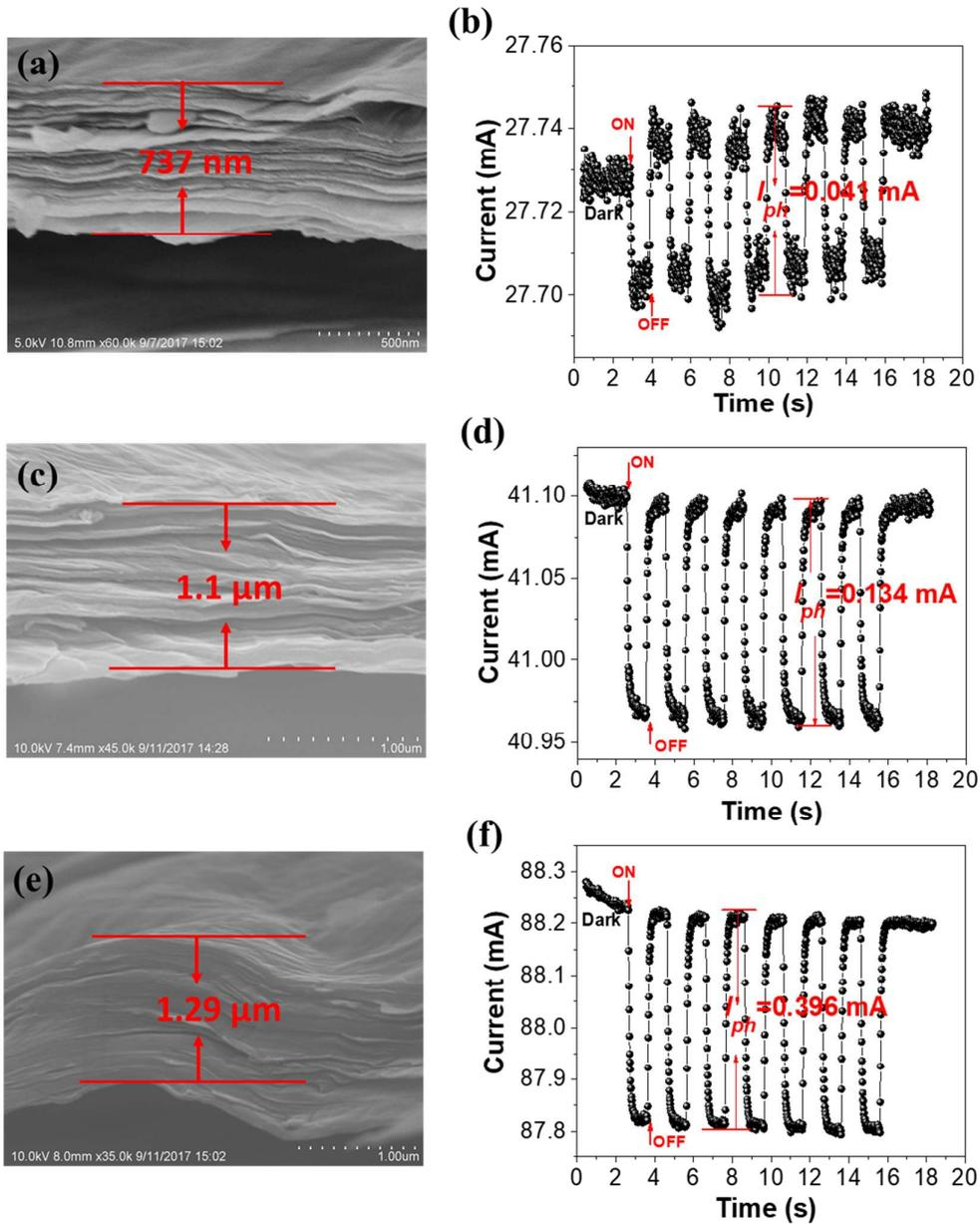
Figure S4: Effects of film thickness on photoresponse. Cross-sectional view SEM images of RGO thin films prepared by (a) four, (c) six and (e) eight drop-casting cycles, respectively and annealing at 1000 °C. (b), (d) and (f) their respective photoresponse measured under laser illumination of 532 nm of 15.1 mW at a bias voltage of 0.5 V. The time interval between two collected data points was set as 13 ms, which is faster than 18 ms in the main text.
