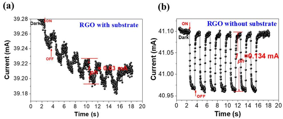
Figure S5: Comparison of photoresponses of fully suspended photodetector with substrate supported photodetector. The RGO thin films prepared by six drop-casting cycles and annealing at 1000 °C. The photoresponse measured under laser illumination of 532 nm of 15.1 mW at a bias voltage of 0.5 V. The time interval between two collected data points was set as 13 ms, which is faster than 18 ms in the main text.
