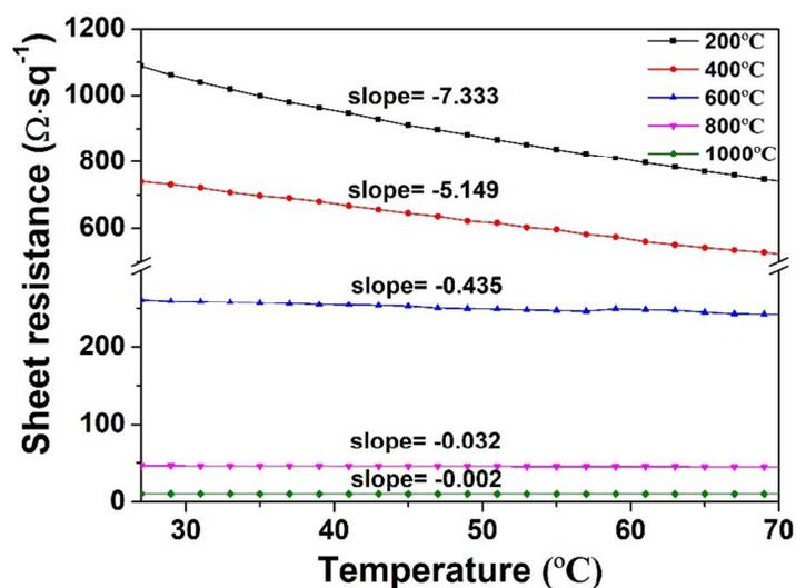
Figure S3: Sheet resistance-temperature plots of RGO thin films prepared at different annealing temperatures measured between 27 °C to 69 °C in vacuum.
