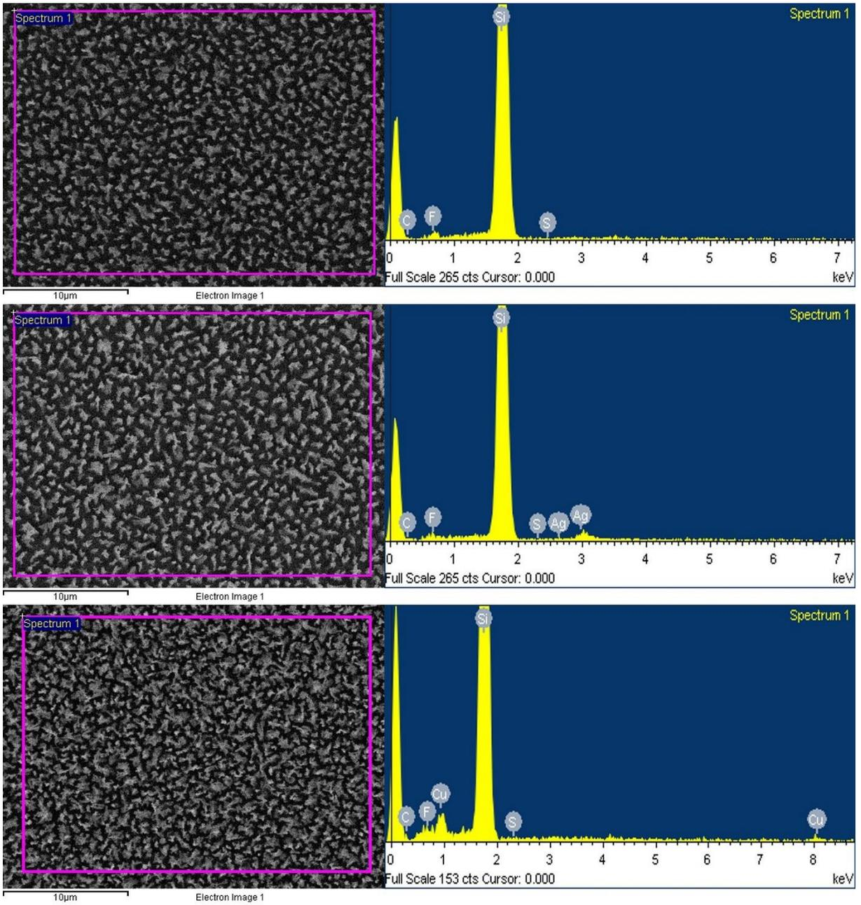
Figure S4: EDAX spectra of NSS, NSS\_Ag and NSS\_Cu surfaces.
