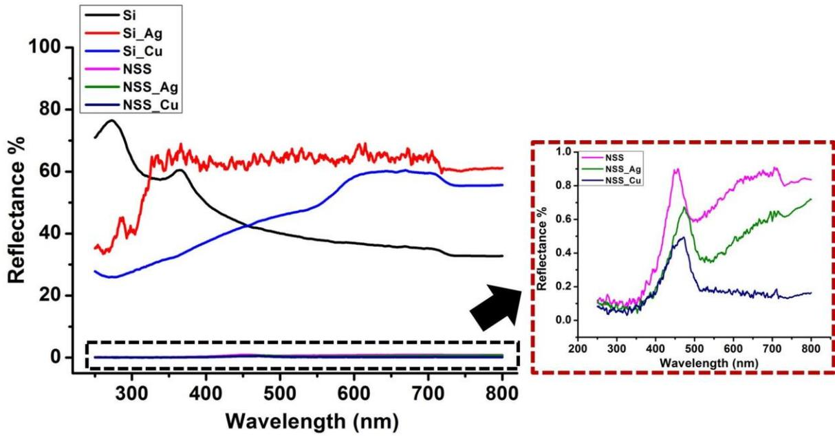
Figure S13: Reflectance Data for all the engineered surfaces with varied wavelength from 250 nm to 800 nm. Inset showing magnified view of reflectance data for only nanostructured surfaces. Reflectance of less than 1% was achieved for the nanostructured surfaces.
