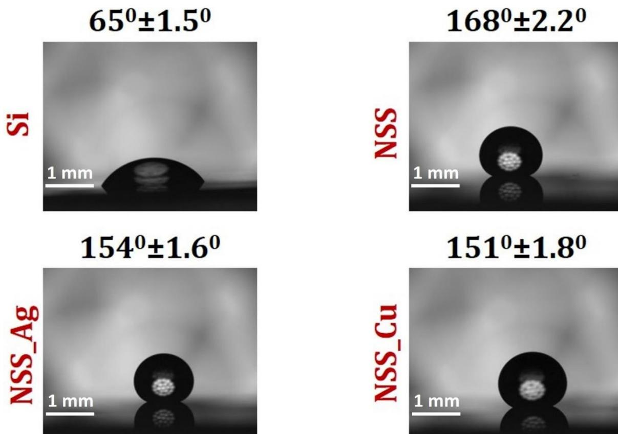
Figure S11: Wettability of all the engineered surfaces: 8  $\mu\text{L}$  droplet was used to measure the static contact angle. NSS, NSS\_Ag and NSS\_Cu exhibited excellent superhydrophobicity with contact angle higher than  $150^{\circ}$  and contact angle hysteresis of less than  $10^{\circ}$  (see Table S2).
