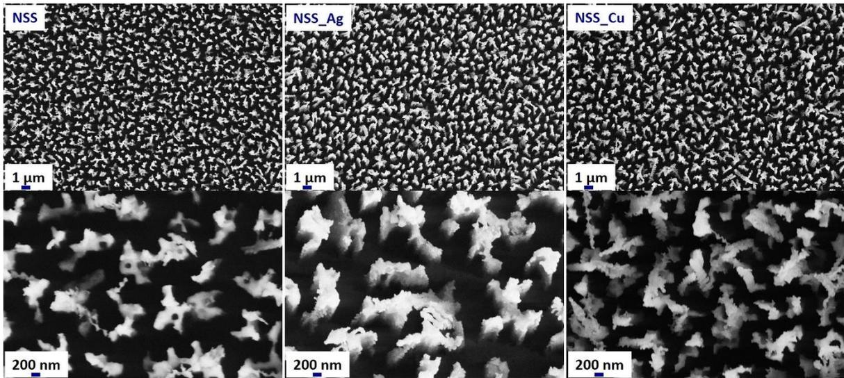
Figure S5: Representative FESEM images of nanostructured surface before and after silver/copper coating.
