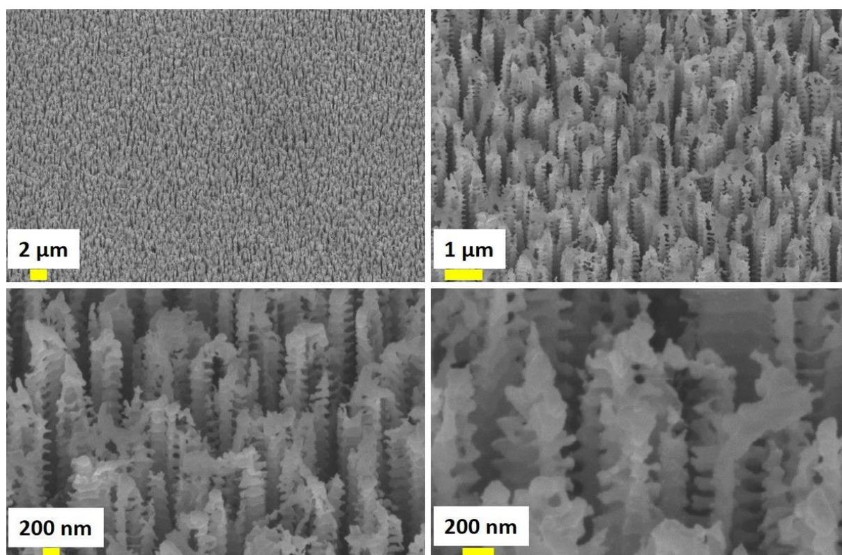
Figure S1: Representative FESEM images of nanostructured surface (45° tilt view) at different magnifications. SEM images show random size and spatial distribution of the nanostructures.
