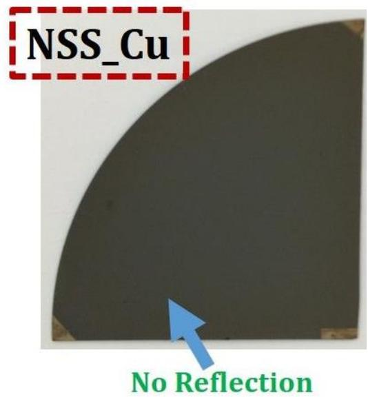
Figure S14: Quarter pieces of silicon and nanostructured surfaces showing reflective and antireflective behaviour respectively. Reflection image of the cell phone is quite clearly seen on the flat silicon surface, whereas no reflection is observed on the nanostructured surfaces.
