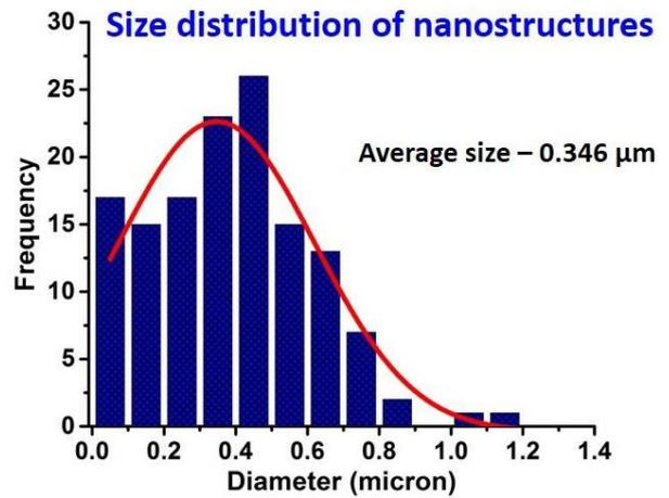
Figure S2: Image J analysis to find the size distribution of the nanostructure base diameter present on the surface. Nanostructures size ranging from 50-1200  $\mu\text{m}$  was observed on the surface with an average diameter of 346 nm.
