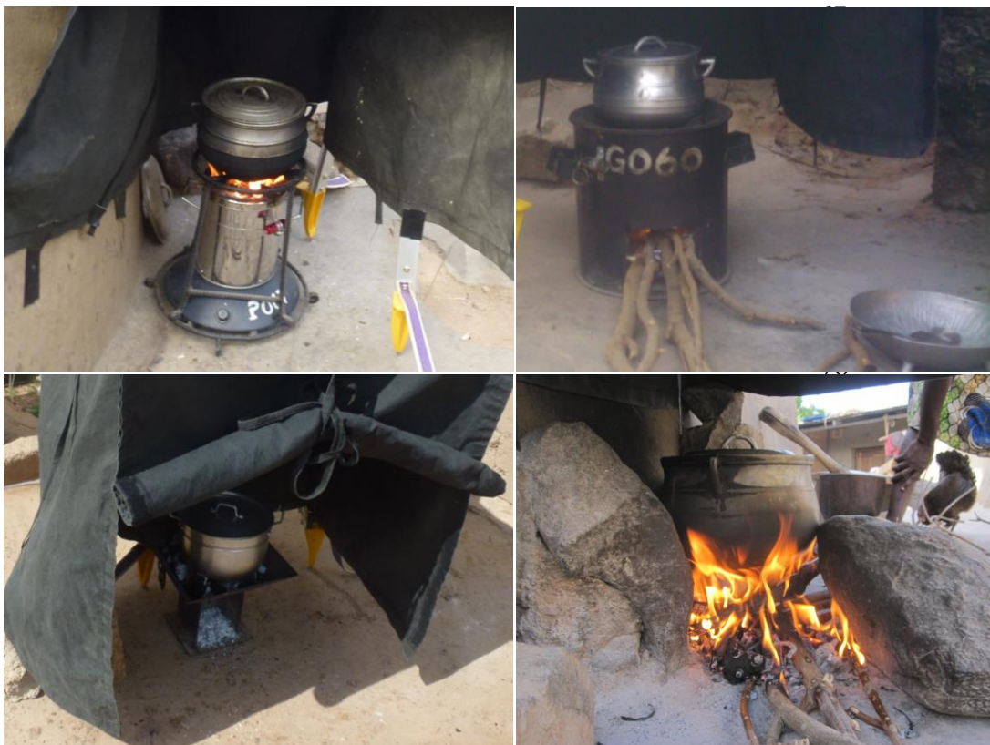
Figure S1: Types of stoves tested in the field (clockwise from top left); Philips HD4012-LS with reinforced pot stand, Gyapa woodstove, threestone fire and local coalpot.
