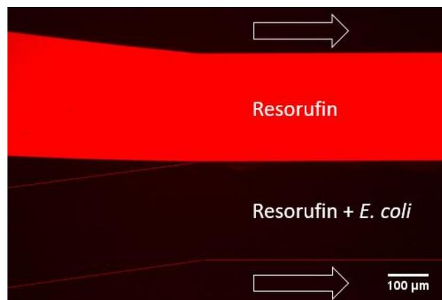
**Figure S3.** Fluorescent image of reactor taken during infusion of resorufin with or without *E. coli*, with arrows indicating flow direction and dashed lines showing the boundary of the channel opposite the nanoporous wall.
