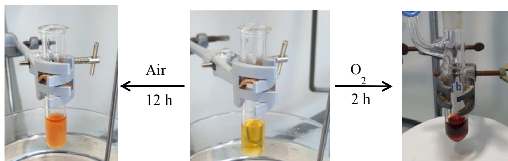
Figure S1. (a) Microwave vessel with NMR analysis of both layers of n BuOH (compound 6 in the red layer, and 4 in the yellow layer of the reaction mixture); (b) Different oxidation time of hydrazine 4 by using air or oxygen in situ .
