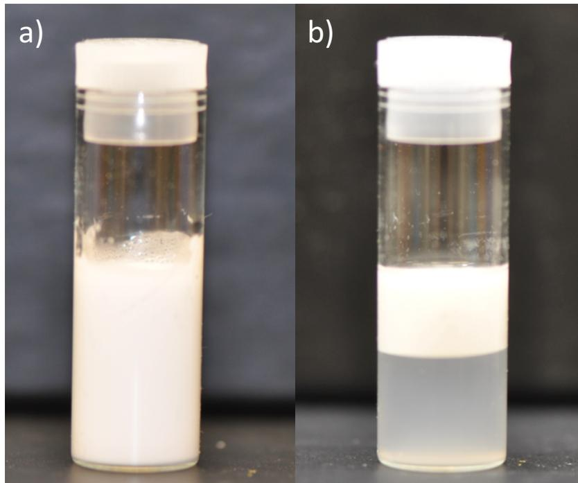
Fig S8. Styrene-in-water emulsions stabilized by mCNC-hexyl<sub>320</sub>-COOH<sub>200</sub> (a) before and (b) after centrifugation.
