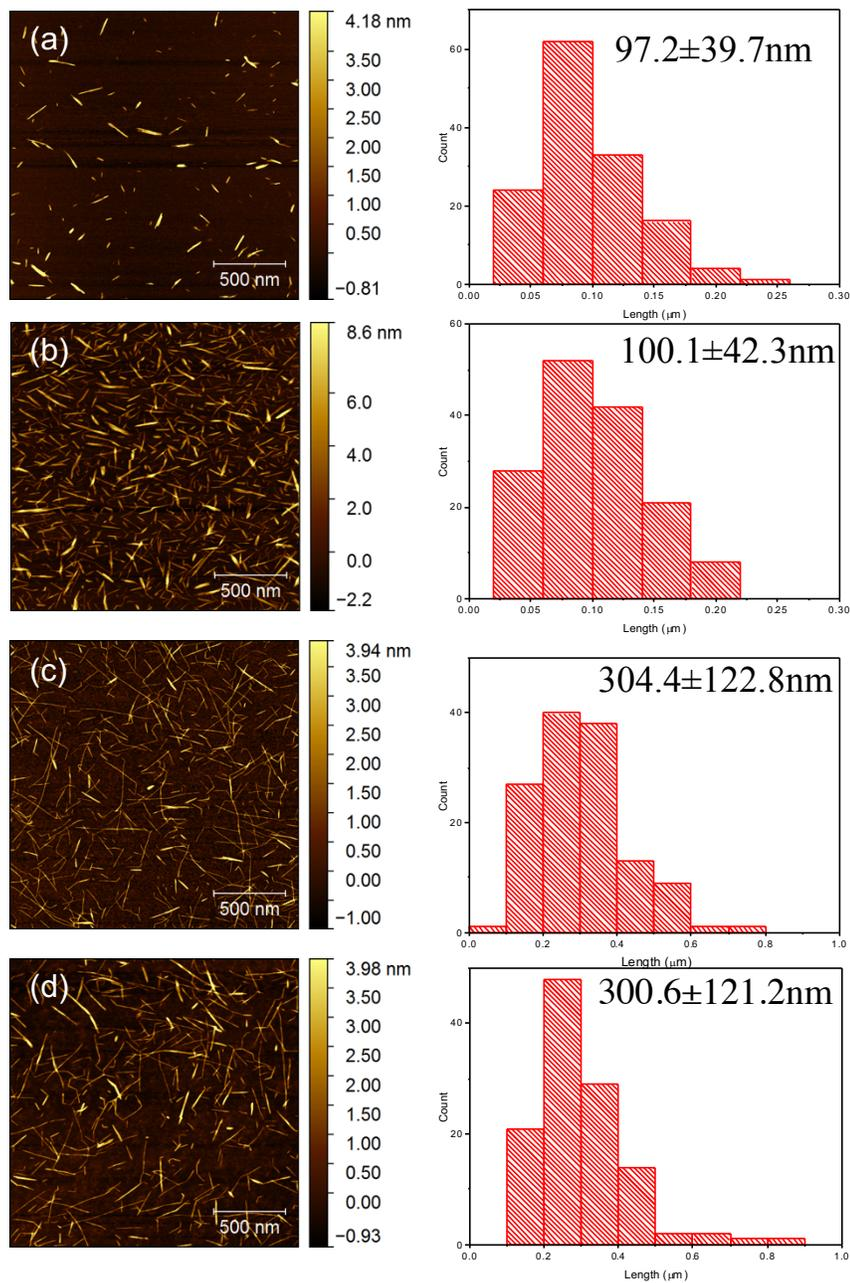
Fig S1. AFM height image of (a) mCNC-COOH<sub>520</sub>, (b) mCNC-hexyl<sub>320</sub>-COOH<sub>200</sub>, (c) MxG-CNC-COOH<sub>920</sub> and (d) MxG-CNC-hexyl<sub>411</sub>-COOH<sub>509</sub>. The average length of each samples measured directly using the image were shown in histogram next to the AFM image.
