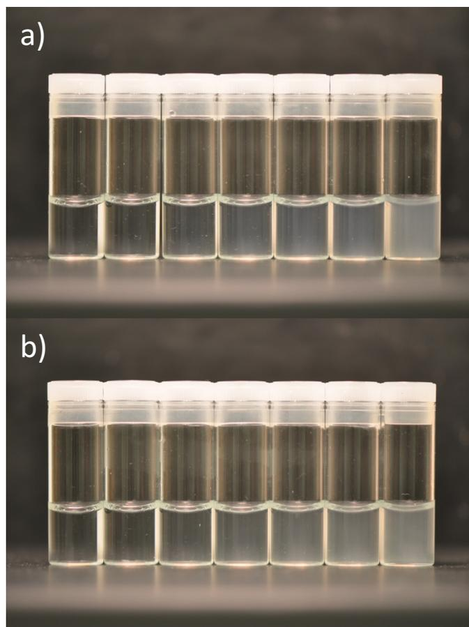
Fig S4. CNC/aqueous dispersion at different concentrations (from left to right, 0.5, 1.0, 2.5, 5.0, 7.5, 10.0 and 15.0 mg/mL) for (a) mCNC-COOH<sub>520</sub> and (b) MxG-CNC-COOH<sub>920</sub>
