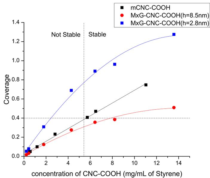
Fig S7. Theoretical coverage versus the effective concentration of CNC-COOH at the interface (i.e. after subtraction of water soluble fraction) per mL of styrene.
