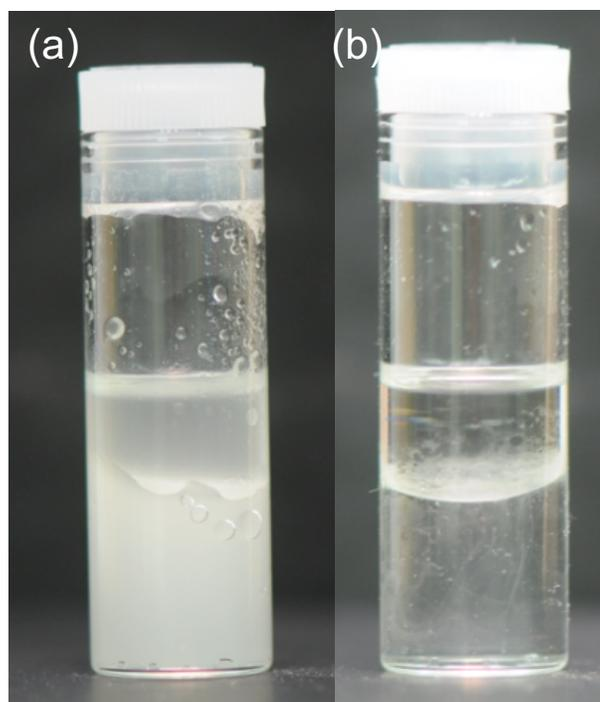
Fig S9. Styrene-in-water emulsions stabilized by 1wt% hexyl amine (a) before and (b) after centrifugation.
