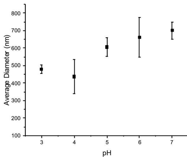
Fig S10. DLS results of the average diameters of the o/w emulsions stabilized by dispersed MxG-CNC-butyl<sub>449</sub>-COOH<sub>471</sub> in phosphate buffer at different pH (the ionic strength of all buffers was set to 50mM by adding additional NaCl).
