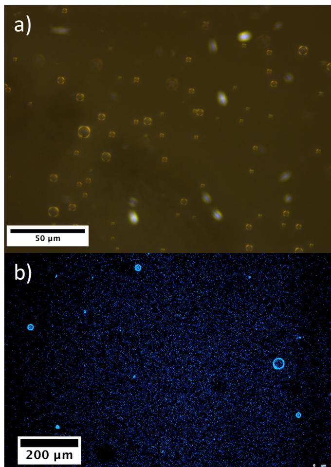
Fig S5. (a) Polarized optical microscope (POM) image and (b) confocal microscope image (with Calcofluor White fluorescence dye added) of the styrene-in-water emulsion stabilized by mCNC-COOH<sub>520</sub>
