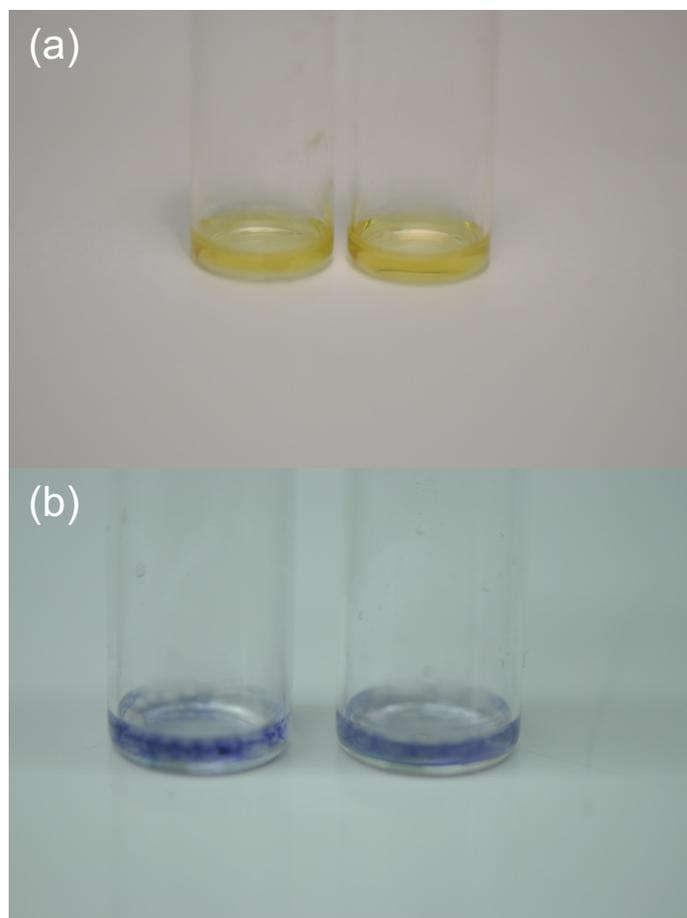
Fig S2. Photographs of the Kaiser test of (a) mCNC-hexyl<sub>320</sub>-COOH<sub>200</sub> (left) and MxG-CNC-hexyl<sub>411</sub>-COOH<sub>509</sub> (right) and (b) mixed sample with hexyl amine and mCNC-COOH<sub>520</sub> (left) and MxG-CNC-COOH<sub>920</sub> (right).
