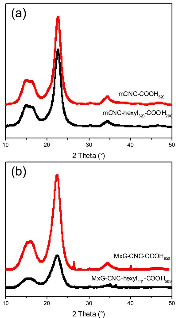
Fig S3. X-ray diffraction pattern of (a) mCNC and (b) MxG-CNC after oxidation (red) and after hydrophobic functionalization with hexyl amine (black).
