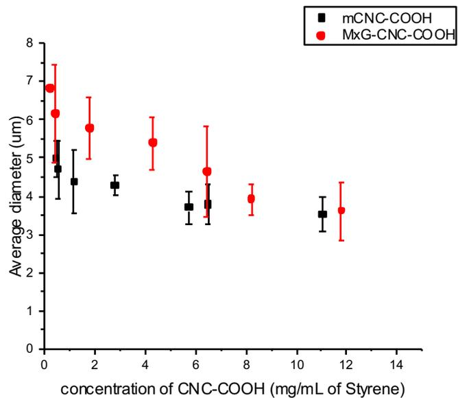
Fig S6. DLS results of the average diameters of the o/w emulsion droplets stabilized by mCNC-COOH<sub>520</sub> and MxG-CNC-COOH<sub>920</sub> versus the effective concentration of CNC-COOH at the interface (i.e. after subtraction of water soluble fraction) per mL of styrene.
