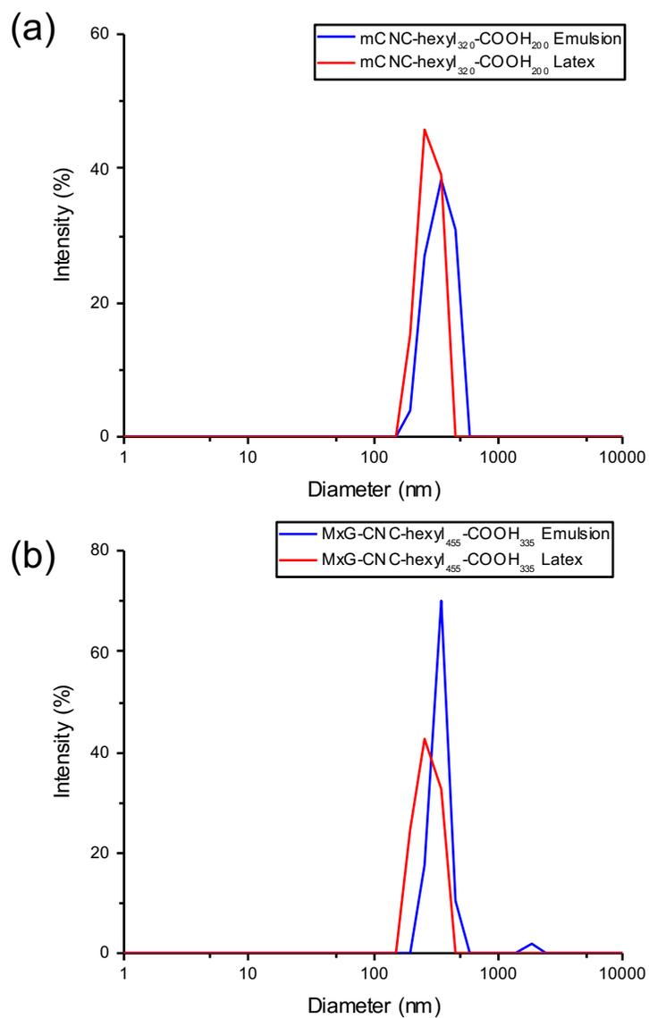
Fig S11. DLS results of the average diameters of the o/w emulsions after sonication and the average diameters of the latex particles after polymerization for (a) mCNC-hexyl<sub>320</sub>-COOH<sub>200</sub> and (b) MxG-CNC-hexyl<sub>455</sub>-COOH<sub>335</sub>.
