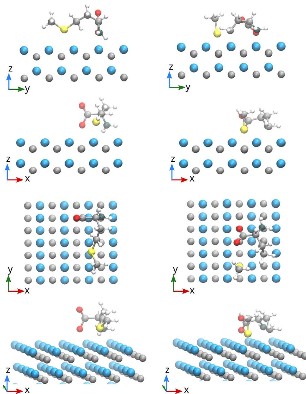
**Figure S3.** Adsorption geometry of an L-methionine conformer (conformer B) on a WC ( $10\bar{1}0$ ) surface before (left) and after (right) atomic relaxation. For simplicity, only part of the simulated metallic slab is shown. Legend: ● = C, ● = N, ● = O, ● = S, ● = W.
