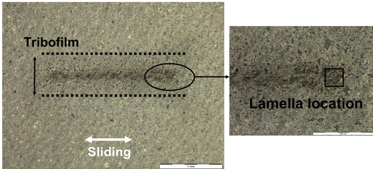
**Figure S7** Stereo microscopy picture of a wear track on a WC functionalized surface after being tested with 1 wt% methionine in glycerol.
