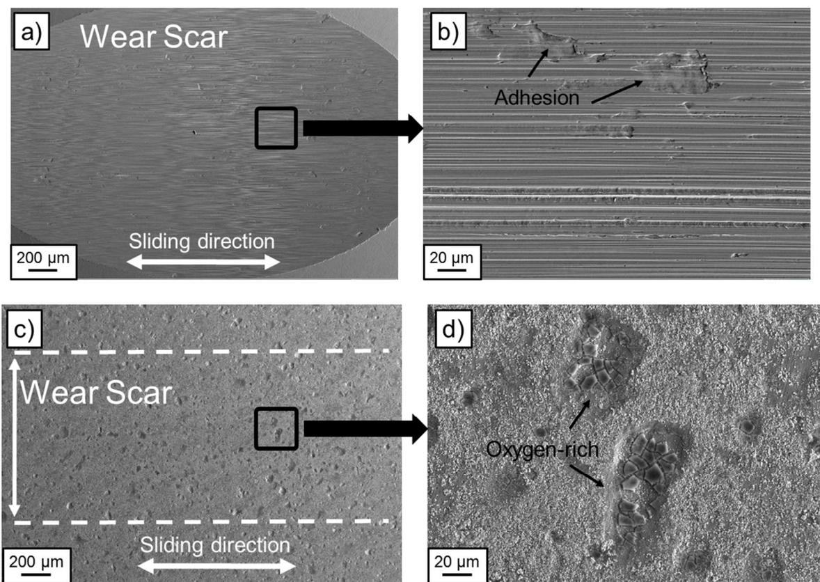
**Figure S6.** Surface topography using secondary electrons of AISI 304 steel surfaces after being tested using a lubricant mixture of 1 wt.% methionine in glycerol (a and b). Surface topography using secondary electrons of functionalized surfaces after being tested using pure glycerol (c and d).
