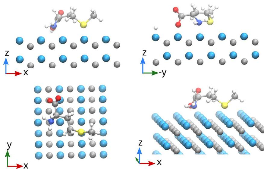
**Figure S2.** Adsorption geometry of an L-methionine conformer (conformer A) on a WC ( $10\bar{1}0$ ) surface. For simplicity, only part of the simulated metallic slab is shown. Legend: ● = C, ● = N, ● = O, ● = S, ● = W.
