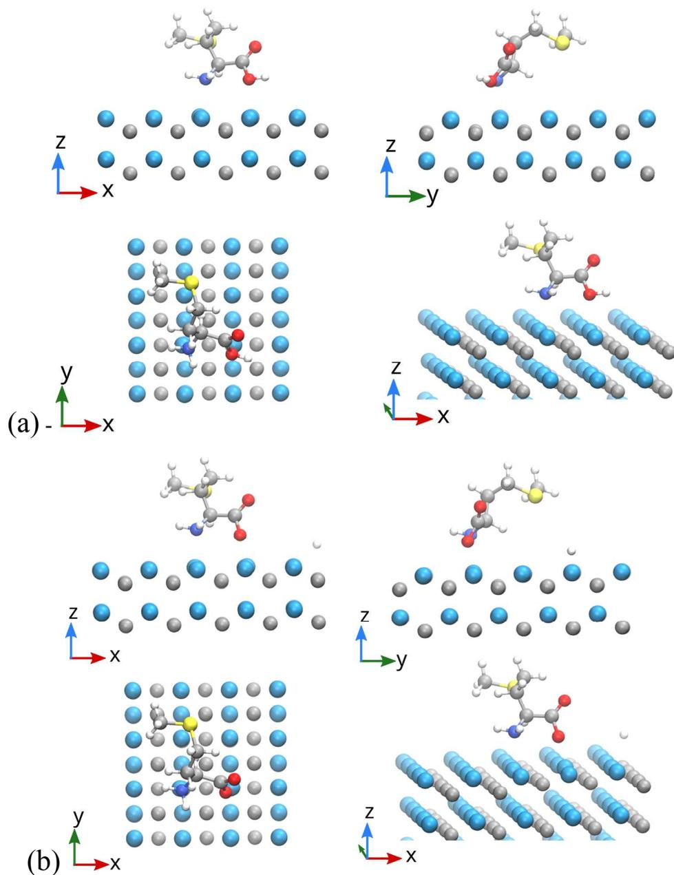
**Figure S1.** Equilibrium adsorption geometry of L-methionine on a WC  $(10\bar{1}0)$  surface (a) and equilibrium adsorption geometry of the dissociated L-methionine on a WC  $(10\bar{1}0)$  surface (b). For simplicity, only part of the simulated metallic slab is shown in both cases. Legend: ● = C, ● = N, ● = O, ● = S, ● = W.
