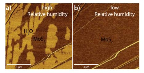
Figure S2: (a) Phase image (tapping mode) of  $MoS_2$  covered with water layers (bright contrast). The water layers were formed when the surface was exposed to  $\sim 75\%$  RH and they disappear when we reduce the RH below 10%, panel (b).
