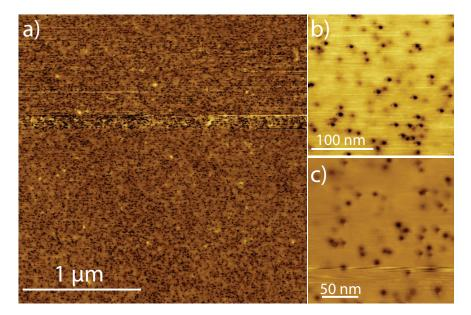
Figure S3: (a) Large scale C-AFM image of  $MoS_2$ . The surface is covered with metal-like defects (dark depressions). (b) A smaller C-AFM image revealing two types of dark defects, deep dark and faint dark depressions. The faint dark depressions are defects in the second  $MoS_2$  trilayer, whereas the deep dark defects are situated in the top  $MoS_2$  trilayer. (c) STM image revealing the same two type of defects with the same contrast variations (setpoint = 0.1 nA and 0.2 V).
