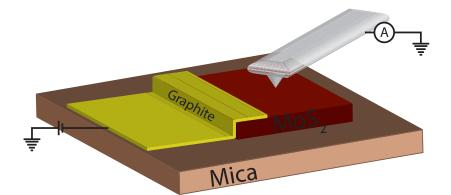
Figure S1: Schematic diagram of the C-AFM configuration. A micrometer thick  $MoS_2$  flake is placed on top of a supporting mica substrate. The mica substrate provides mechanical stability. A large graphite flake (millimeters wide) makes electrical contact with the  $MoS_2$ .
