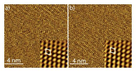
Figure S5: (a-b) Consecutive LFM images of  $MoS_2$  obtained with 20 nN tip load. Both images clearly show stick and slip motion with atomic periodicity that matches the lattice constant of  $MoS_2$ . insets: atomic scale low pass filtered images of the respective LFM images, showing a clear hexagonal symmetry with a periodicity of 0.31 nm, i.e., close to the  $MoS_2$ lattice constant.
