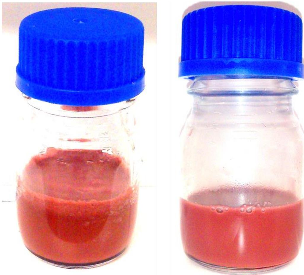
**Figure S7:** Cu nanowire based nanofluids: After 1 washing (L) and after 2 washings (R). The excess residual HDA is evident from whitish coloured froth in fluid after 1 washing.
