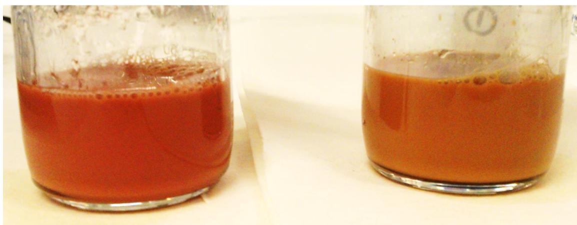
**Figure S8:** Copper nanowire based nanofluid (Left) after 2 washings and re-dispersion with PVP and ascorbic acid and (R) with excessive washings (3-4). The brick red colour of the nanofluid after three washings turned to yellowish brown within a week along with rapid deterioration in thermal conductivity.
