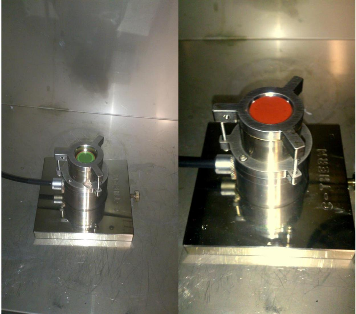
**Figure S4:** C-Therm thermal conductivity analyser-modified transient plane source method: Sensor assembly, and sensor assembly with Cu nanofluid sample.
