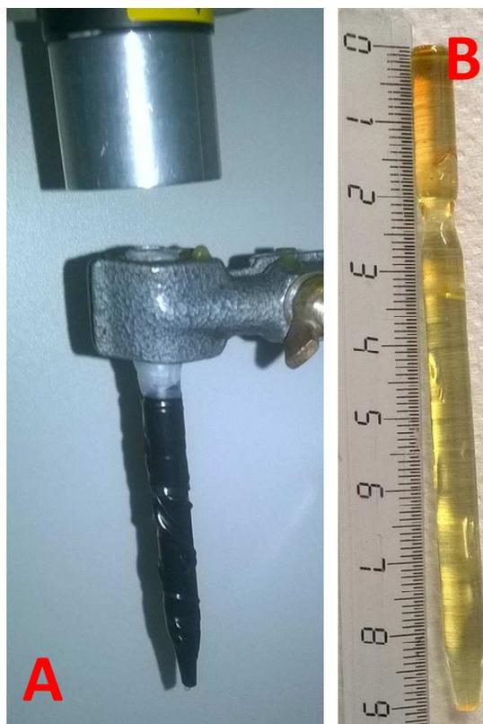
**Figure S2: A:** Experimental set-up used for the photopolymerization of the model resin (thickness = 9 cm) (LED@405 nm); Pasteur pipette **wrapped in black tape** with polymerizable medium containing: 0.13 wt% of Cu(I) / 2.0 wt% Iod / 6 wt% Tin(II). B: **9 cm cured polymer after breaking the glass (Pasteur Pipette) surrounding the polymer**
