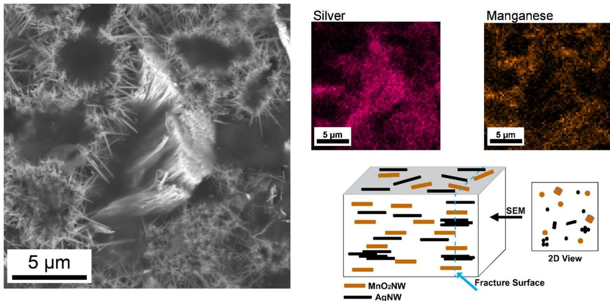
Figure S2: SEM image of the fracture surface of 2.0vol% AgNW/1.0vol% MnO<sub>2</sub>NW/PMMA hybrid nanocomposite with elemental analysis map.
