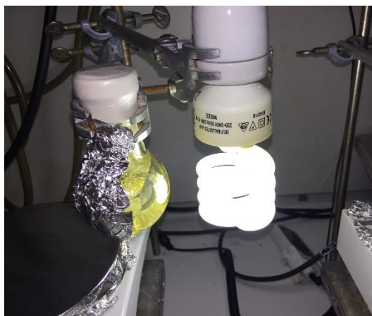
Figure S1: Setup for irradiations on a preparative scale under irradiation with a 25 W energy-saving UV/vis CFL bulb.
