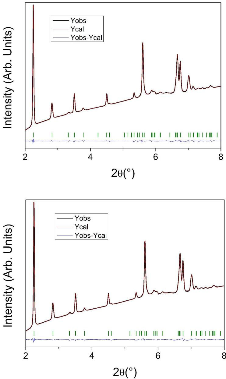
**Figure S1.** Low-angle region ( $2^\circ$ - $8^\circ$ ) of the experimental (black), calculated (red) and difference (blue) profiles obtained from the Rietveld refinement of the  $P2_1$  structure ( $R_p=11.8\%$ ,  $R_{wp}=4.4\%$ ,  $R_{Bragg}=6.2\%$ ) (top) and the  $Pbn2_1$  structure ( $R_p=12.2\%$ ,  $R_{wp}=4.6\%$ ,  $R_{Bragg}=6.0\%$ ) of TON at 1.56(2) GPa (bottom). Vertical bars indicate the calculated positions of the Bragg reflections.
