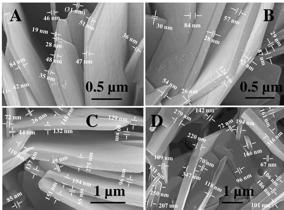
**Figure S3.** (A-D) Close-up side view of THE large smooth nanoplates obtained at 180 min and measurements of the nanoplate thicknesses. Concentration of  $\text{AgNO}_3$  precursor: 5 M.
