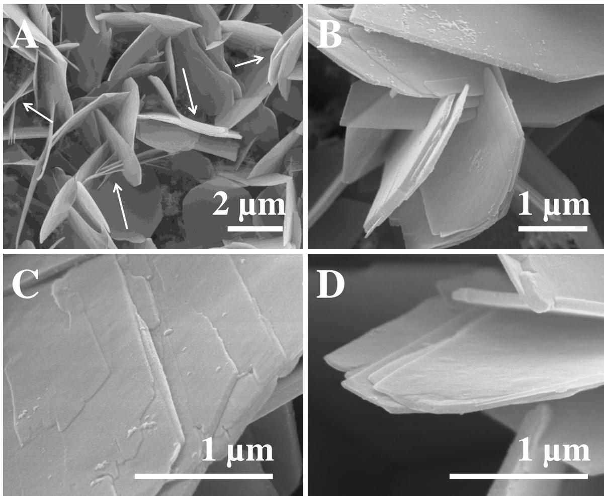
**Figure S2.** SEM characterization reveals polymerization of the large nanoplates. Growth time: (A) 130 min, (B) 150 min, (C) 160 min, and (D) 180 min.
