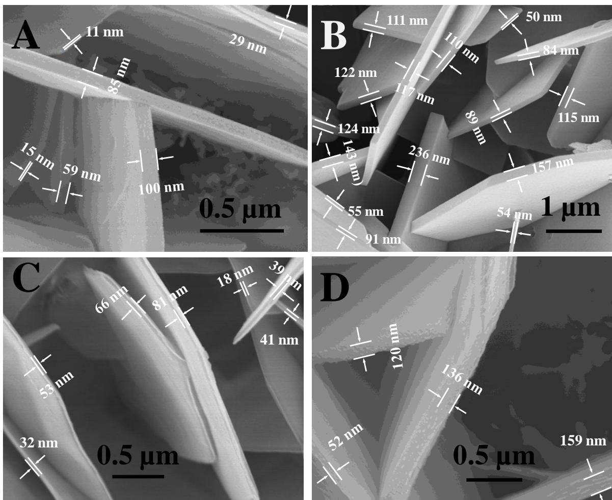
**Figure S4.** (A-D) Close-up side view of the large smooth nanoplates obtained at 180 min and measurements of the nanoplate thicknesses. Concentration of  $\text{AgNO}_3$  precursor: 1 M.
