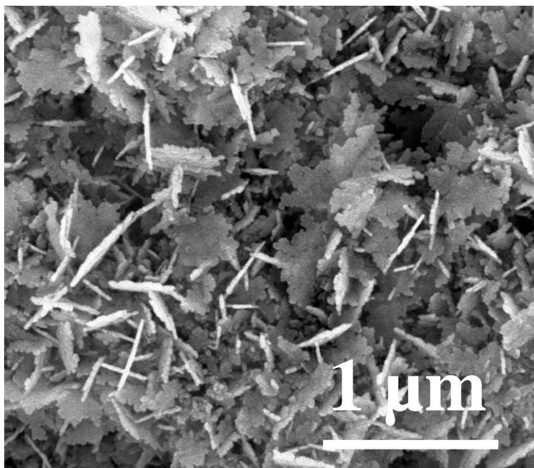
**Figure S1.** Small nanoplates with rough surfaces and ragged edges grown from a 0.1M AgNO<sub>3</sub> aqueous solution after UV illumination for 180 min.
