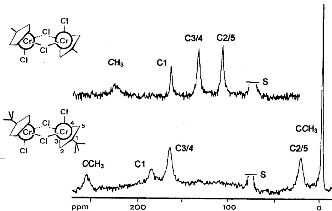
**Figure S1.**  $^{13}\text{C}$  NMR spectra of  $[(\text{MeCp})\text{CrCl}_2]_2$  at 337 K and  $[(t\text{-BuCp})\text{CrCl}_2]_2$  at 305 K both dissolved in  $\text{CDCl}_3$  (S).
