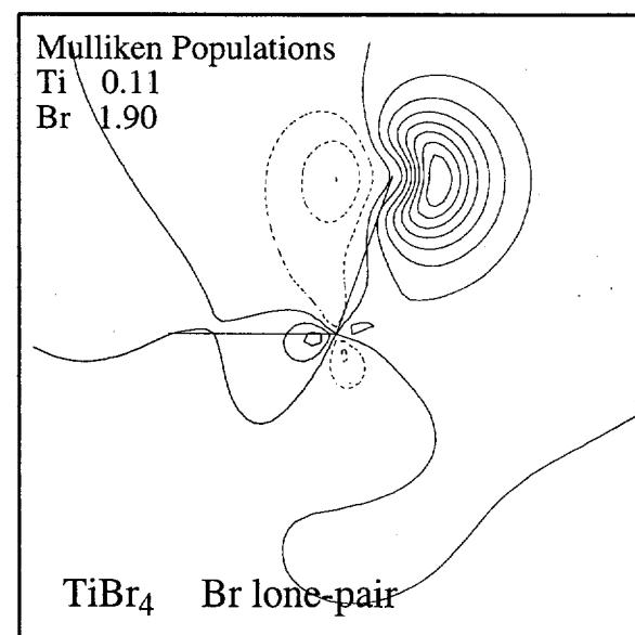
**S1.** LMO plots of Ti-X  $\sigma$ -bonds and X lone-pairs in TiX<sub>4</sub> (X=F,Br).
