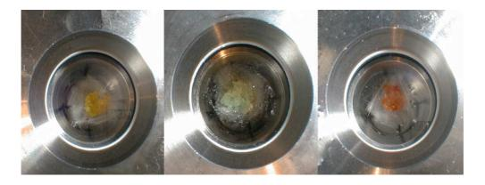
Color change of polymer-supported catalyst **1b** during the hydroformylation of *cis*-2-butene in a batch system. (i) Initial yellow color of **1b**. (ii) Pale yellow of  $RhH(CO)_2(BINAPHOS)$  (**5**). (iii) Red color due to the formation of a new species.
