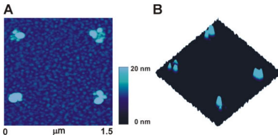
**Figure 2.** Zoom-in image of two component protein pattern after reaction with anti-IgG. (A) Topography image and (B) phase image
