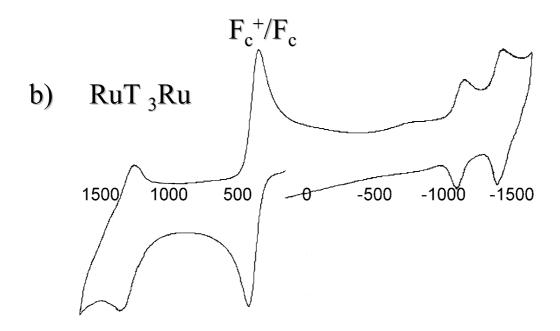
Figure S1: Cyclic voltammetry in 0.1 M TBAPF<sub>6</sub>/CH<sub>3</sub>CN solution and 0.1 M concentration 1.0 x  $10^{-4}$  M for the RuT<sub>3</sub> and 2.5 x  $10^{-3}$  M for RuT<sub>3</sub>Ru. Potentials were measured at a Pt working electrode referenced to a Pt wire quasi-reference electrode. Potentials were standardized using a ferrocene (Fc) internal reference and are converted to SCE scale assuming that E<sub>1/2</sub> (Fc/Fc<sup>+</sup>) = 0.38 V.
