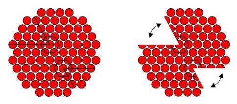
As for the n-gonal defects, the disclination is created by cutting-off one sector (and only one) of  $60^{\circ}$  in the n juxtaposed hexagons. Then, the cone forms by joining the two cut-edges of each hexagons leaving n pentagons (here, two pentagons).
