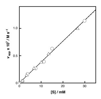
**Figure S4.** Plot of  $v_{app}$  against the substrate concentration for the reaction of p-ClC<sub>6</sub>H<sub>4</sub>OH ( $\bigcirc$ ) and of p-ClC<sub>6</sub>D<sub>4</sub>OH ( $\triangle$ ).
