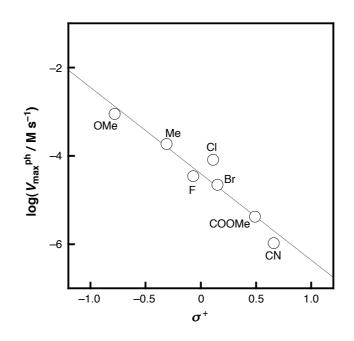
*Figure S3.* Hammett plot for the oxygenation of phenols by oxy-hemocyanin (single turnover reaction); data are taken from Table 1).
