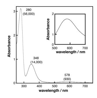
*Figure S11.* UV-vis spectrum of oxy-hemocyanin from *Octopus vulgaris* (5.5 x  $10^{-5}$  M) taken in 0.1 M Tris-HCl buffer (pH 7.4) at 25 °C under O<sub>2</sub>-saturated conditions. Inset: Magnified spectrum (1.9 x  $10^{-3}$  M).
