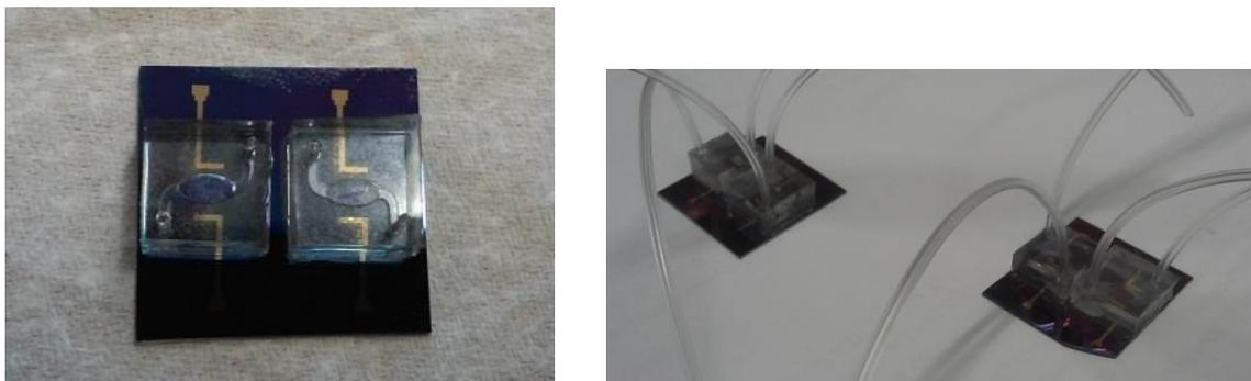
**Figure. S1** Photographs of polydimethylsiloxane (PDMS) microfluidic device with integrated electrodes (left) and the chamber in its assembled form.
