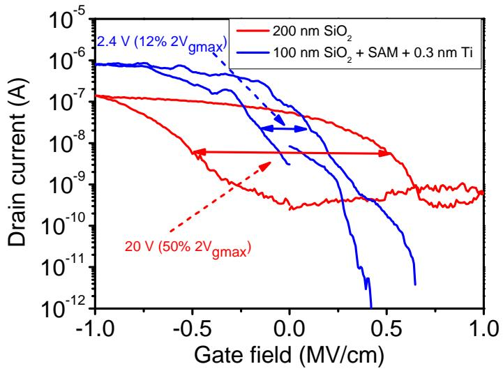
**Figure S3** Transfer curve of two devices: In red a SWCNT FET with a  $200\text{ nm SiO}_2$  dielectric. In blue a SWCNT FET with a  $100\text{ nm SiO}_2$  and a SAM on top. The hysteresis in this case is only 12% of the gate voltage window (determined by the difference between the minimum and maximum gate voltage) at a gate voltage sweep rate of  $0.38\text{ V/s}$  ( $3.8 \times 10^4\text{ V/cm s}$ ).
