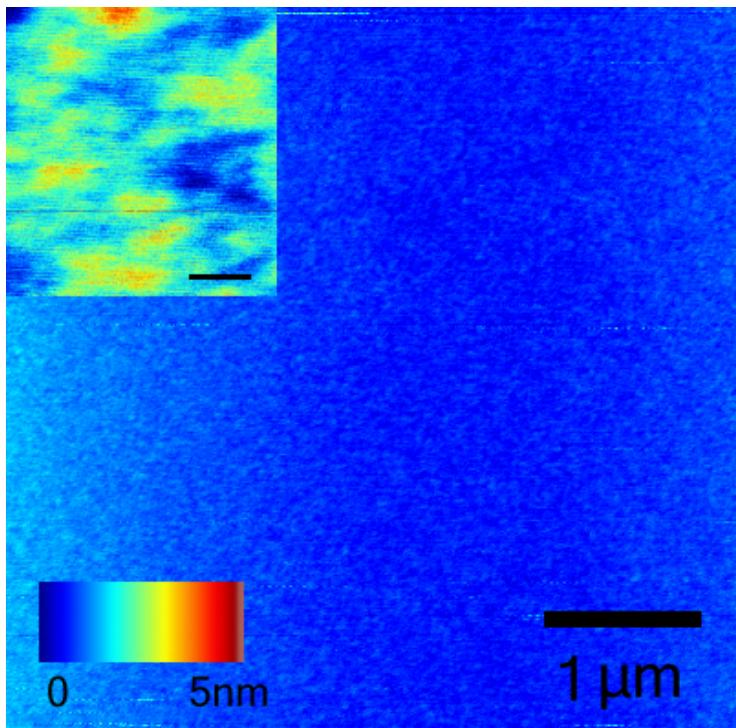
**Figure S1** Tapping-mode atomic force microscopy (AFM) image of the silicon substrate covered by the SAM. The layer is very smooth and pinhole free across large areas. **Inset** Zoom. The scale bar here is 20 nm, and the colour scale ranges from 0 to 0.5 nm.
