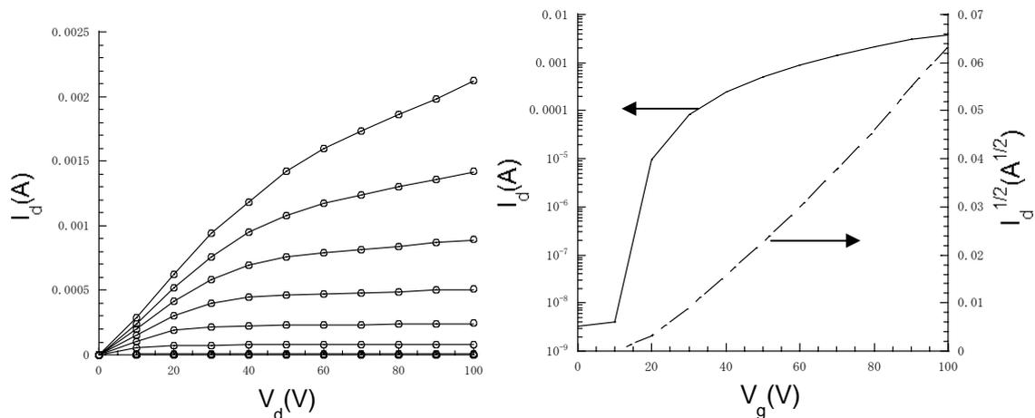
**Figure S9.** Output and transfer characteristic of **2b (black)** with bottom-contact geometry.
