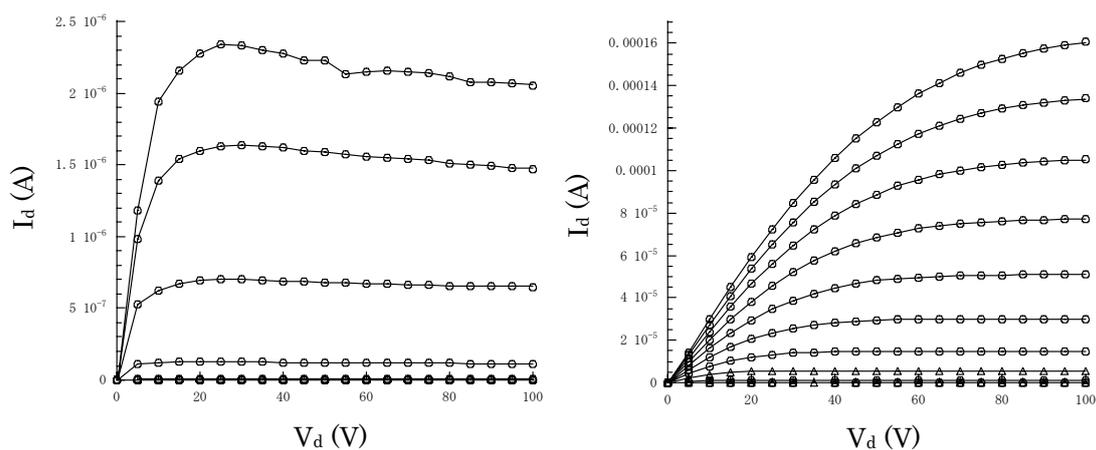
**Figure S10.** Output characteristics of **1b** and **2b (black)** with top-contact geometry.
