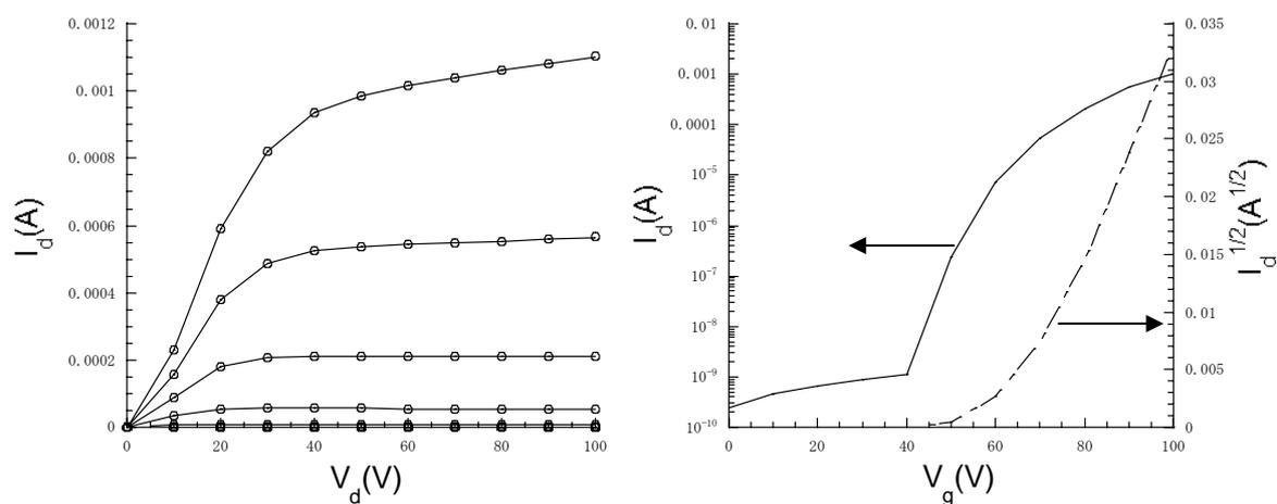
**Figure S7.** Output and transfer characteristic of **1d** with bottom-contact geometry .
