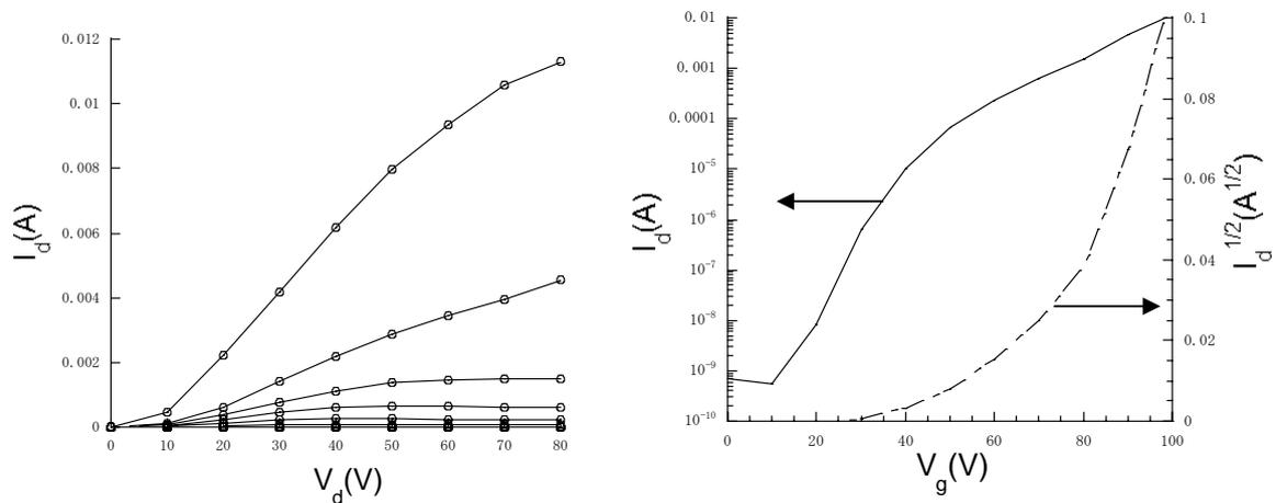
Figure S5. Output and transfer characteristic of **1b** with bottom-contact geometry.
