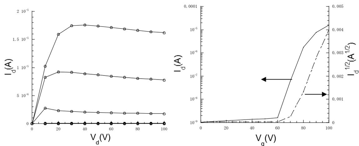
**Figure S8.** Output and transfer characteristic of **2a** with bottom-contact geometry.
