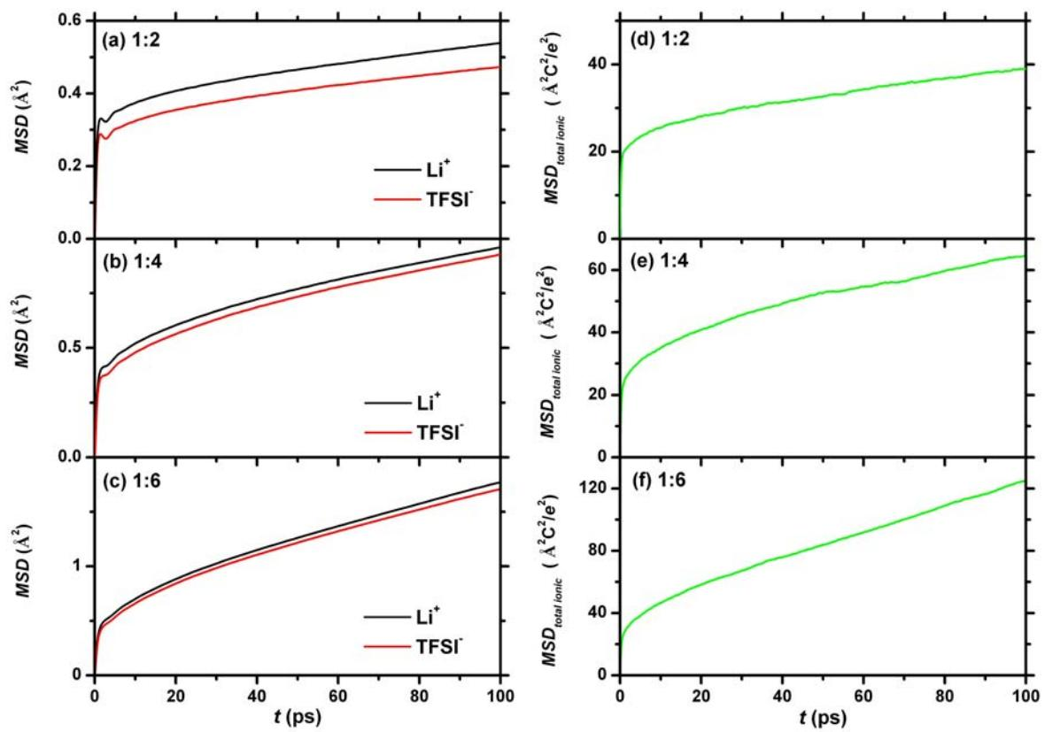
Fig. 11. Ionic mean square displacement (MSD) (left column) and total ionic MSD (right column), respectively, for (a), (d) LiTFSI1-ACE<sub>2</sub>; (b), (e) LiTFSI1-ACE<sub>4</sub>; and (c), (f) LiTFSI1-ACE<sub>6</sub>; black for the Li<sup>+</sup> ion, red for the TFSI<sup>-</sup> ion, and green for the total ionic MSD. In the right column,  $e=1.6022\times 10^{-19}$  C, i.e. unit electron charge.
