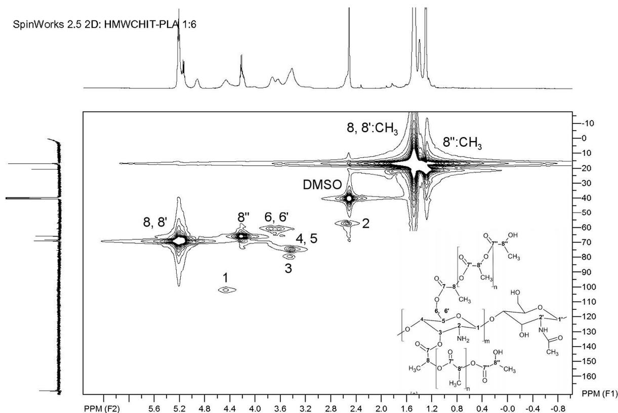
**Figure S4.** HMQC spectrum of HMWCHIT-PLA 1:6 sample, after 4 hours of reaction at 40 °C. Peak assignments are the same as on Fig. S3.
