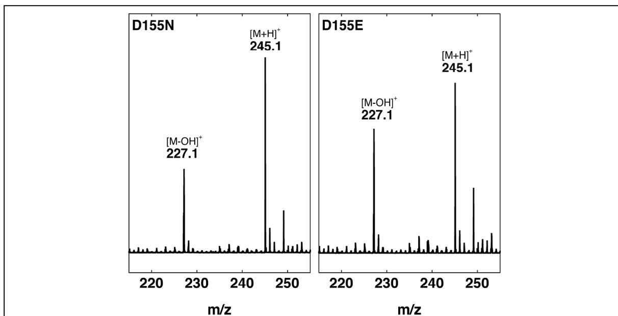
Figure S3. Mass spectrum of biotin observed in two BioB mutant proteins' final reaction mixtures. The catalytic activity of BioB proteins was measured under standard assay conditions. After acid precipitation of the proteins, the reactionary products present in the sample mixtures were detected using ESI-MS. Both the Asp155Asn and Asp155Glu mutants do not show a detectable level of biotin by HPLC, however, these samples do show trace amount of biotin by ESI-MS, as shown
