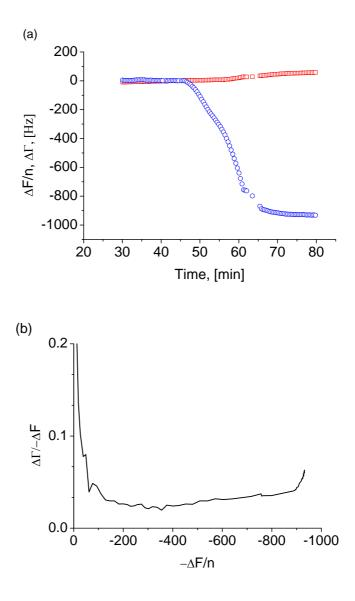
Figure S1: Formation of a pNIPAM gel on a gold-coated QCM crystal by electrochemically induced free radical polymerisation.
