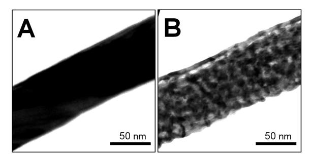
**Figure S1.** TEM image of  $Au_{0.65}/Ag_{0.35}$  alloy NRs (A) before and (B) after chemical ethcing.
