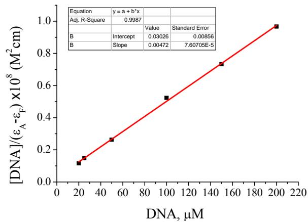
**Figure S7.** Binding constant curve fit. Compound **1** binding to poly(dN)<sub>25</sub>.
