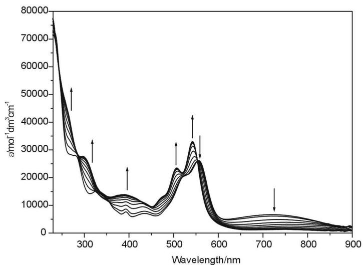
**Figure S10.** UV-visible spectra recorded in  $\text{CH}_2\text{Cl}_2$  containing  $[\text{Bu}_4\text{N}][\text{BF}_4]$  (0.4 M) using spectroelectrochemical methods for **3** at 273 K showing the interconversion of **3** to **3**<sup>2+</sup>. Arrows indicate the progress of the oxidation.
