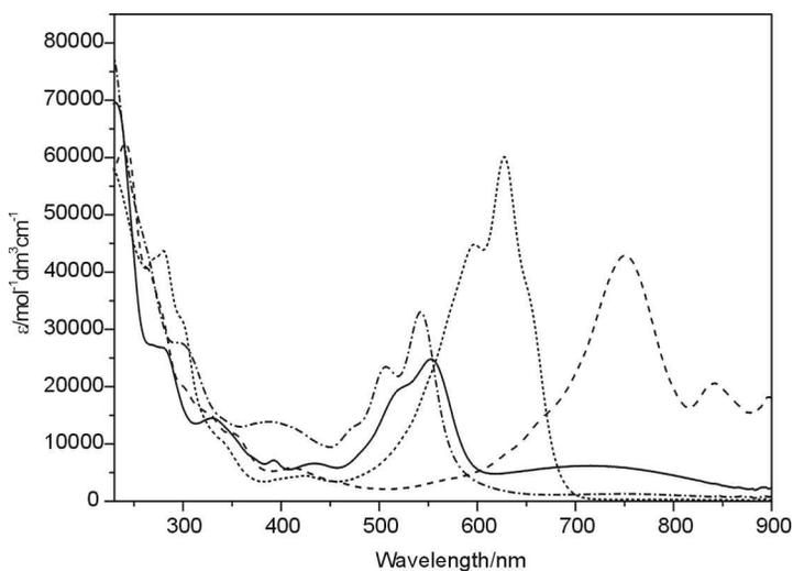
**Figure S6.** UV-visible spectra recorded in  $\text{CH}_2\text{Cl}_2$  containing  $[\text{Bu}_4\text{N}][\text{BF}_4]$  (0.4 M) using spectroelectrochemical methods for **3** at 273 K. The spectrum of **3** is represented by the solid line,  $3^-$  (dashed line),  $3^{2-}$  (short dashed line) and the oxidised species  $3^{2+}$  recorded at 243 K (dashed-dotted line)
