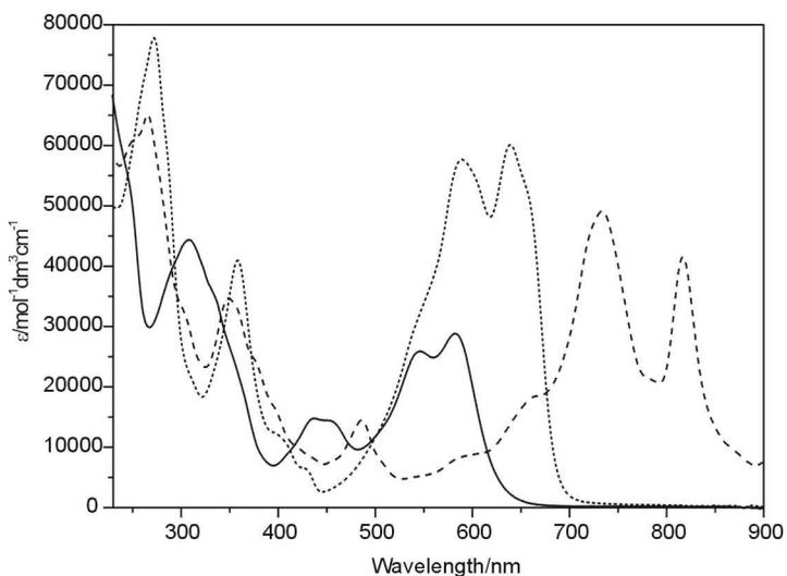
**Figure S7.** UV-visible spectra recorded in CH<sub>2</sub>Cl<sub>2</sub> containing [Bu<sub>4</sub>N][BF<sub>4</sub>] (0.4 M) using spectroelectrochemical methods for **5** at 273 K. The spectrum of **5** is represented by the solid line, **5<sup>•+</sup>** (dashed line) and **5<sup>2+</sup>** (short dashed line).
