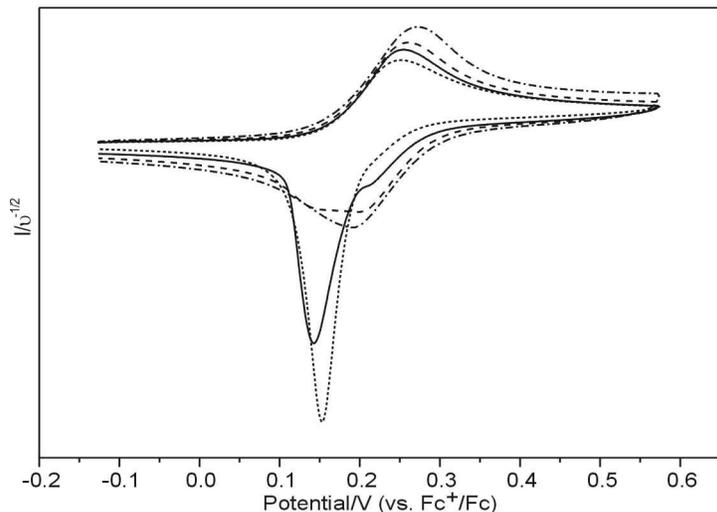
**Figure S1** Cyclic voltammograms recorded for **1a** in CH<sub>2</sub>Cl<sub>2</sub> containing [Bu<sub>4</sub>N][BF<sub>4</sub>] (0.4 M) showing the effect of scan rate on profile of the oxidation process. 0.02 Vs<sup>-1</sup> (short dashed line), 0.10 Vs<sup>-1</sup> (solid line), 0.20 Vs<sup>-1</sup> (dashed line), and 0.50 Vs<sup>-1</sup> (dashed-dotted line).
