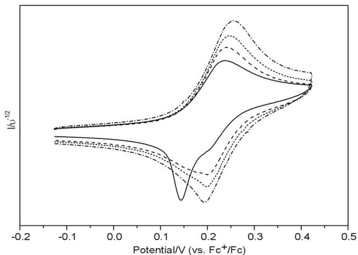
**Figure S2.** Cyclic voltammograms recorded for **1a** in CH<sub>2</sub>Cl<sub>2</sub> containing [Bu<sub>4</sub>N][BF<sub>4</sub>] (0.4 M) showing the effect of scan rate on profile of the oxidation process. 0.10 Vs<sup>-1</sup> (solid line), 0.50 Vs<sup>-1</sup> (dashed line), 1.00 Vs<sup>-1</sup> (short dashed line) and 2.00 Vs<sup>-1</sup> (dashed-dotted line).
