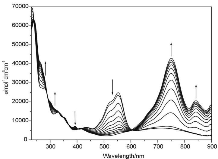
**Figure S8.** UV-visible spectra recorded in CH<sub>2</sub>Cl<sub>2</sub> containing [Bu<sub>4</sub>N][BF<sub>4</sub>] (0.4 M) using spectroelectrochemical methods for **3** at 273 K showing the inter-conversion of **3** to **3<sup>•+</sup>**. Arrows indicate the progress of the reduction.
