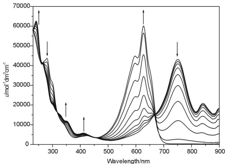
**Figure S9.** UV-visible spectra recorded in  $\text{CH}_2\text{Cl}_2$  containing  $[\text{Bu}_4\text{N}][\text{BF}_4]$  (0.4 M) using spectroelectrochemical methods for **3** at 273 K showing the inter-conversion of **3** to **3**<sup>2-</sup>. Arrows indicate the progress of the reduction.
