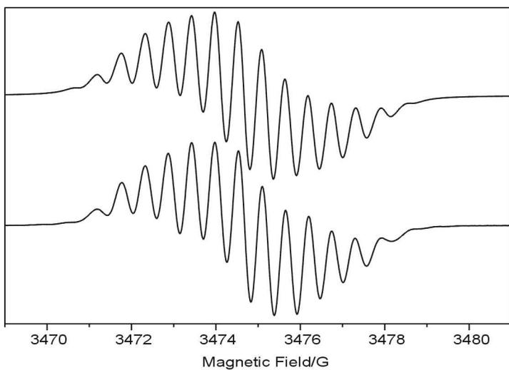
**Figure S3.** Experimental (bottom) and simulated (top) EPR spectra for electrochemically generated **1a<sup>-</sup>** in CH<sub>2</sub>Cl<sub>2</sub> containing [Bu<sub>4</sub>N][BF<sub>4</sub>] (0.4 M) at 291 K.
