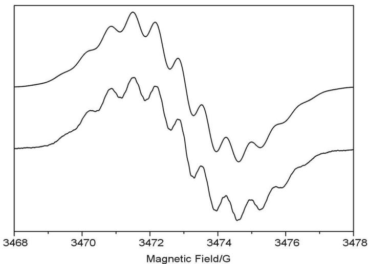
**Figure S4.** Experimental (bottom) and simulated (top) EPR spectra for electrochemically generated **2<sup>-</sup>** in CH<sub>2</sub>Cl<sub>2</sub> containing [Bu<sub>4</sub>N][BF<sub>4</sub>] (0.4 M) at 291 K.
