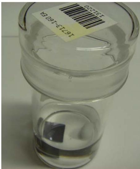
**Figure S4:** Picture of the reactor setup employed for the on chip chemistry. The silicon wafer and the stir bars are at the bottom of the reactor dipped in water with 17-25 mM 4-nitrobenzene diazonium water and 1 wt% SDS.
