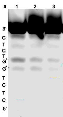
Figure S6. Polyacrylamide gel electrophoresis (PAGE) pattern of 5'-FAM-end-labeled duplex 1 (0.5 \mu M) without or with Cu-Pt complex. Lane 1, ODN I; Lane 2, ODN I + 1 \mu M complex 4 ; Lane 3, ODN I + 1 \mu M complex 3 . The faded bands of G*G* in the presence of complex suggest that some GG has been platinated by the complex, which decreases the formic acid-catalyzed depurination and thus the subsequent cleavage by piperidine (V. Brabec, M. Leng, Proc. Natl. Acad. Sci. USA 1993 , 90, 5345-5349).
