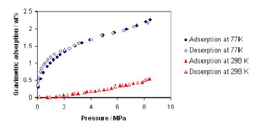
**Figure S9:** Hydrogen adsorption and desorption isotherms at 77K and at 298K for bis[(trimethylsilyl)methyl]Cr-HMS after hydrogenation.
