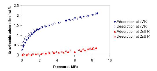
**Figure S8:** Hydrogen adsorption and desorption isotherms at 77K and at 298K for bis[(trimethylsilyl)methyl]Cr-HMS before hydrogenation.
