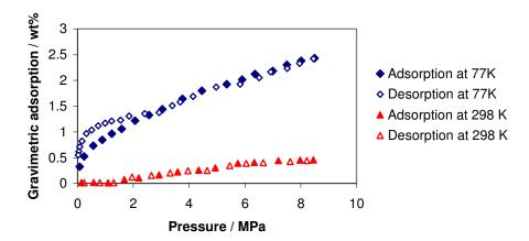
**Figure S5:** Hydrogen adsorption and desorption isotherms at 77K and at 298K for tris(mesityl)V-HMS after hydrogenation.
