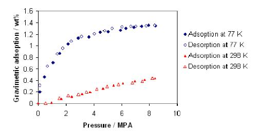
Figure S1: Hydrogen adsorption and desorption isotherms at 77K and at 298K for plain silica (HMS).
