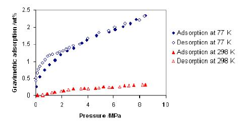
**Figure S4:** Hydrogen adsorption and desorption isotherms at 77K and at 298K for tris(mesityl)V-HMS before hydrogenation.
