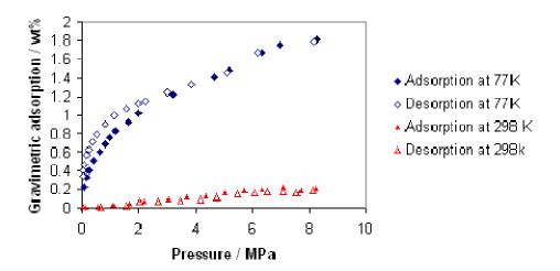
**Figure S6:** Hydrogen adsorption and desorption isotherms at 77K and at 298K for tris[bis(trimethylsilyl)methyl]Cr-HMS before hydrogenation.
