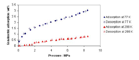
Figure S2: Hydrogen adsorption and desorption isotherms at 77K and at 298K for tetra(benzyl)Ti-HMS.
