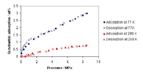
**Figure S3:** Hydrogen adsorption and desorption isotherms at 77K and at 298K for bis(naphthalene)Ti-HMS.
