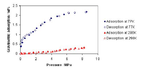
**Figure S7:** Hydrogen adsorption and desorption isotherms at 77K and at 298K for tris[bis(trimethylsilyl)methyl]Cr-HMS after hydrogenation.
