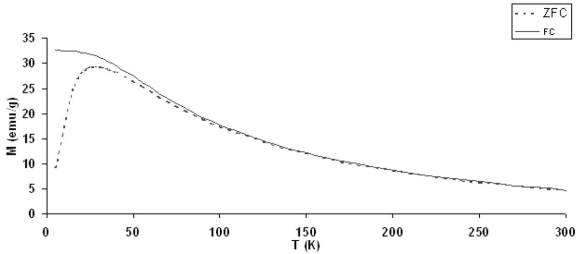
**Fig. 6S.** Field-cooled (FC) and Zero-field-cooled (ZFC) magnetizations of MG NPs versus temperature measured in a field of 100 Oe.
