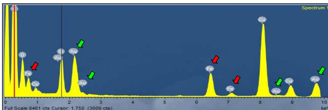
**Figure 2S.** EDX spectra of Fe<sub>3</sub>O<sub>4</sub>@Au (lactose)<sub>50</sub> (Linker)<sub>50</sub> nanoparticles: green arrows (Au peaks) and red arrows (Iron peaks).
