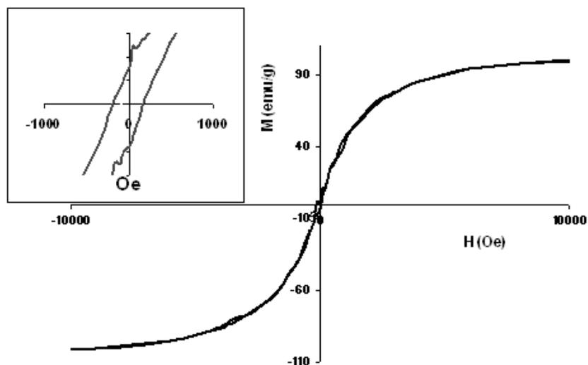
**Fig. 5S.** Magnetization (emu per gram of Fe) versus applied field curve measured at 300K of the MGPNs. Inserted image: the corresponding hysteresis curve measured at 5K.
