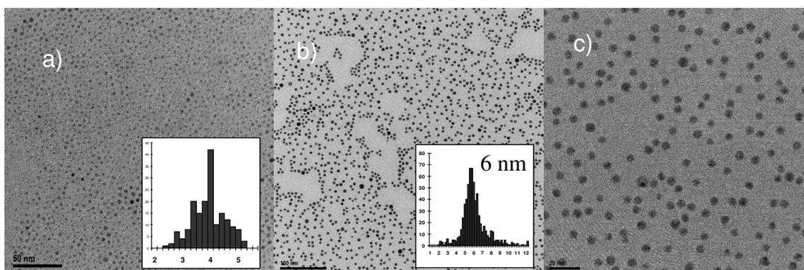
**Figure 1S.** TEM images of a) Fe<sub>3</sub>O<sub>4</sub>(oleic) nanoparticles (4 nm) and b) and c) Fe<sub>3</sub>O<sub>4</sub>@Au(oleic) nanoparticles (6 nm).
