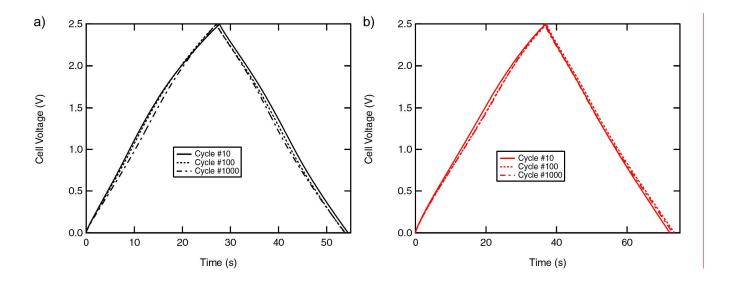
Figure S3. Charge/discharge cycles (#1, #10, #1000) of lifetime testing at 1A/g. a) as-prepared composite. b) oxidized composite.
