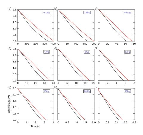
**Figure S1.** Constant current discharge profiles of as-prepared composite (black curves) and oxidized composite (red curves). a) discharge at 0.1A/g. b) discharge at 0.2A/g. c) discharge at 0.5A/g. d) discharge at 1A/g. e) discharge at 2A/g. f) discharge at 5A/g. g) discharge at 10A/g. h) discharge at 20A/g. i) discharge at 50A/g.
