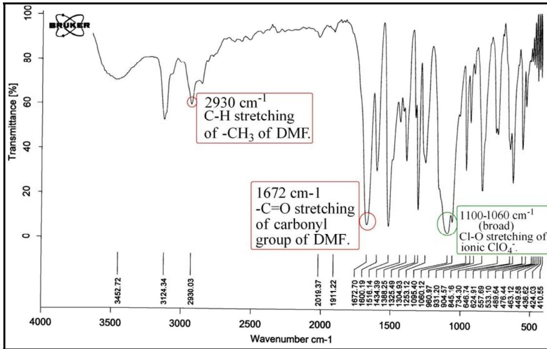
**Figure S5.** FTIR spectrum of as synthesized compound **2**.
