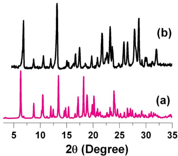
**Figure S20.** PXRD patterns of (a) simulated pattern of **2a**. (b) experimental pattern of **2a**.
