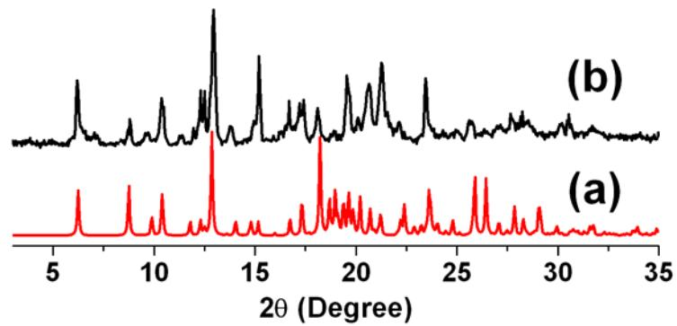
**Figure S16.** PXRD patterns of (a) simulated pattern of **1**. (b) experimental pattern of **1**.
