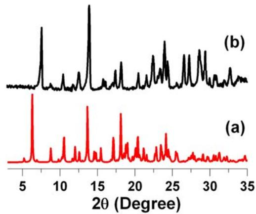
**Figure S21.** PXRD patterns of (a) simulated pattern of **2b**. (b) experimental pattern of **2b**.
