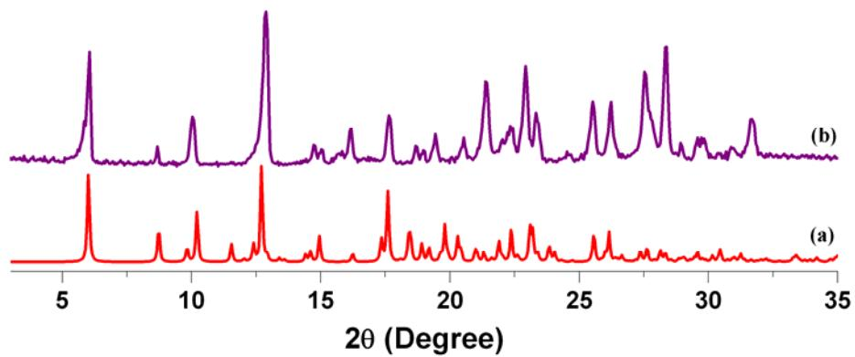
**Figure S18.** PXRD patterns of (a) simulated pattern of **3**. (b) experimental pattern of **3**.
