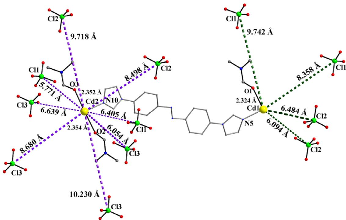
**Figure S24.** Crystal structures of compound **2a**, showing the distances between Cd(II) and Cl Atoms of  $\text{ClO}_4^-$  anions.
