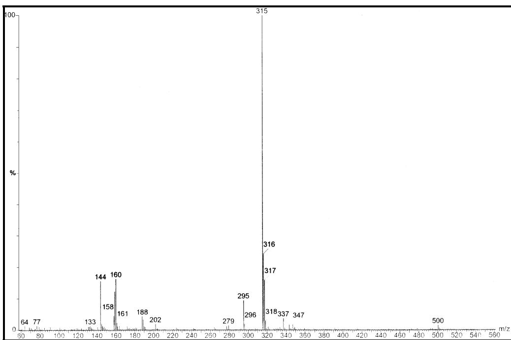
**Figure S2.** ESI mass spectrum of ligand azim (bis-(4-imidazol-1-yl-phenyl)-diazene).
