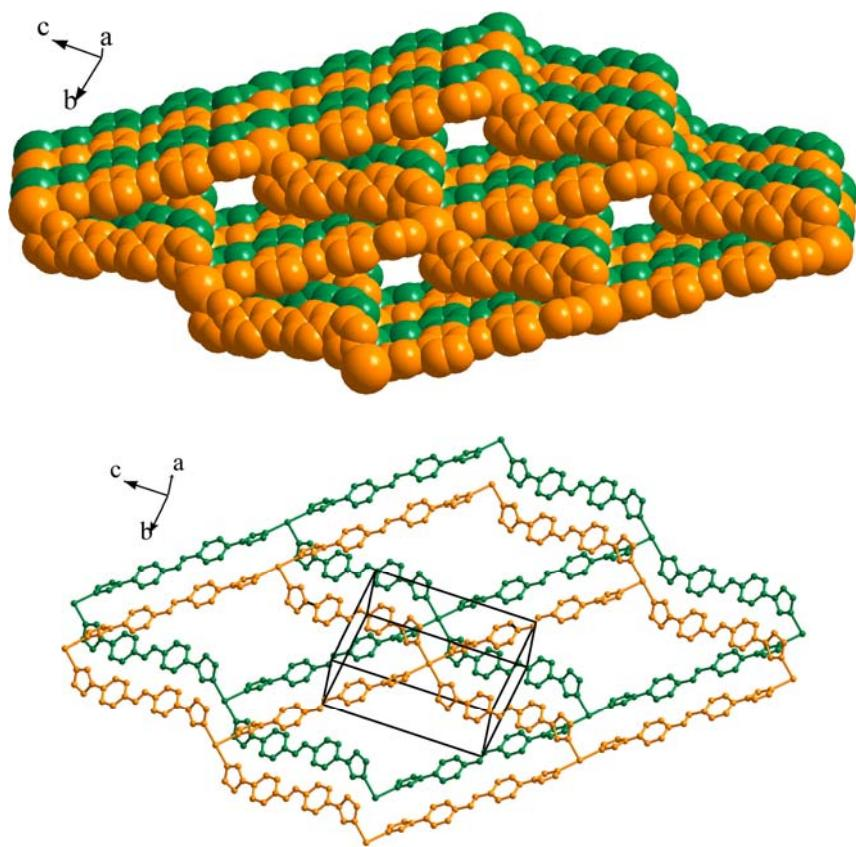
**Figure S27.** A view of **1** (top) showing ABAB....stacking mode of grid layers (CPK model). 2D rhombus grid networks of **1** (bottom) with cell edges (guest molecules are removed for clarity).
