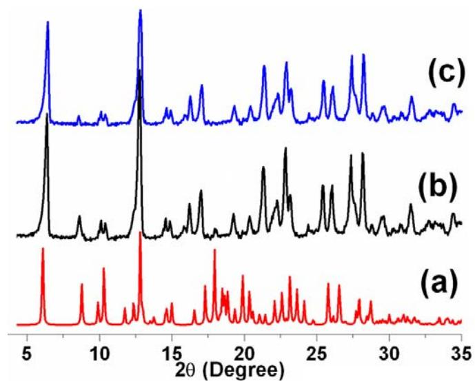
**Figure S17.** PXRD patterns of (a) simulated pattern of **2**. (b) experimental pattern of **2**.
