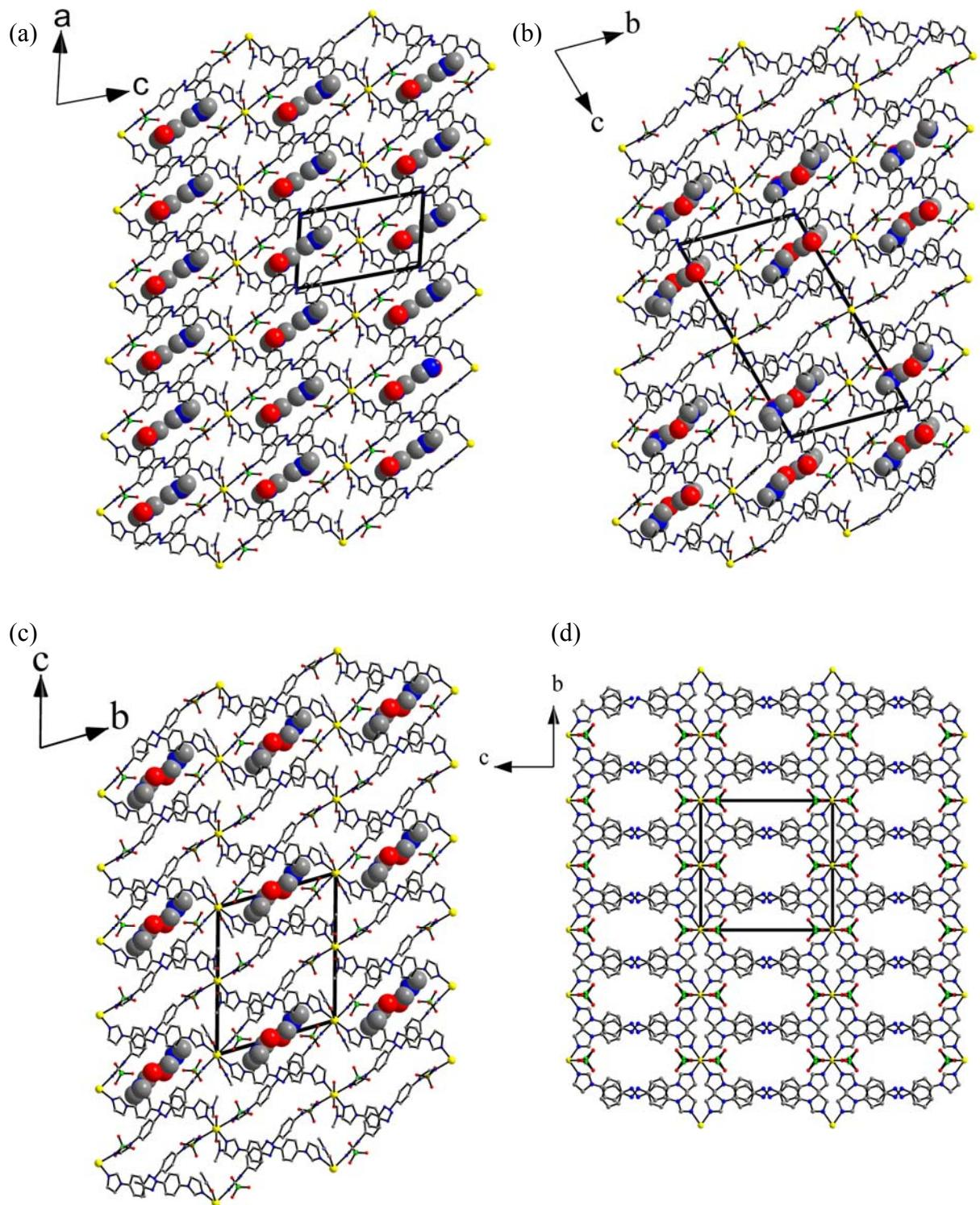
**Figure S28.** Crystal structure of **2** (a), **2a** (b), **2b**(c) and **2c** (d). Cd, pale yellow; O, red; N, blue; C, gray; Cl, green; (grid networks in stick mode showing guest DMF molecules in space-filling mode)
