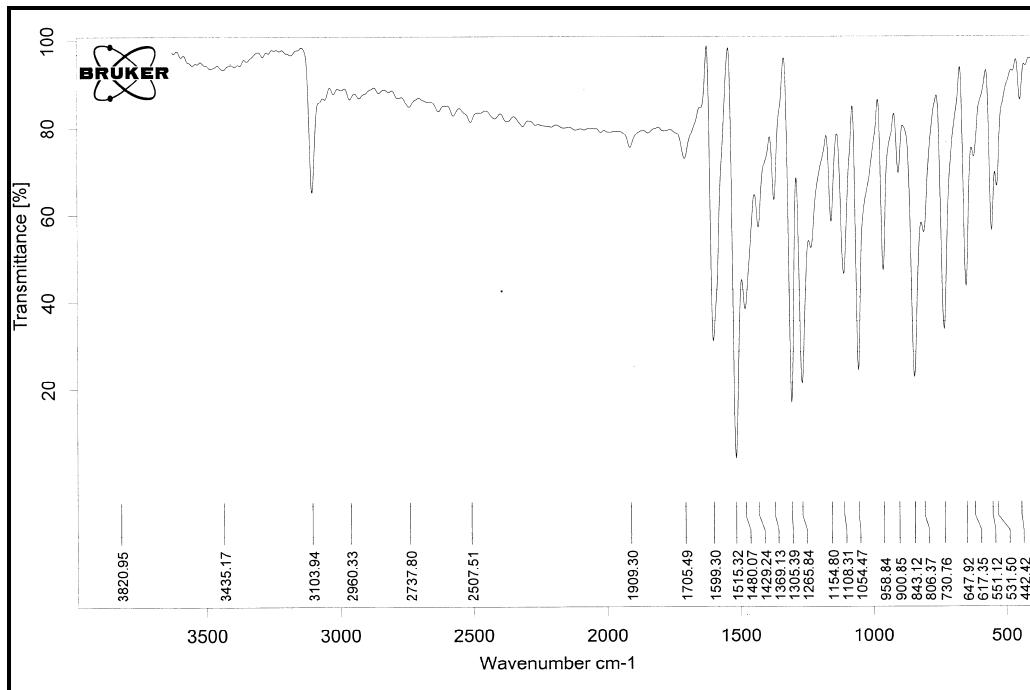
**Figure S1.** FTIR spectrum of ligand azim (bis-(4-imidazol-1-yl-phenyl)-diazene).
