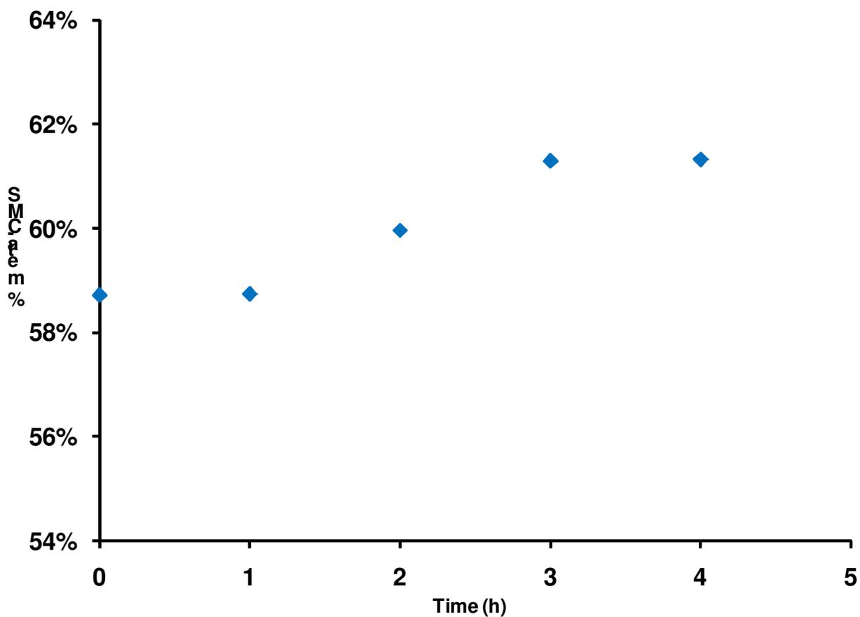
**Figure S1.** Percentage of meta-CMS monomer present in polymerization process during run 7.
