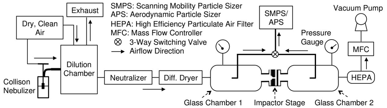
Figure S1. Experimental setup for the impaction stage evaluation.
