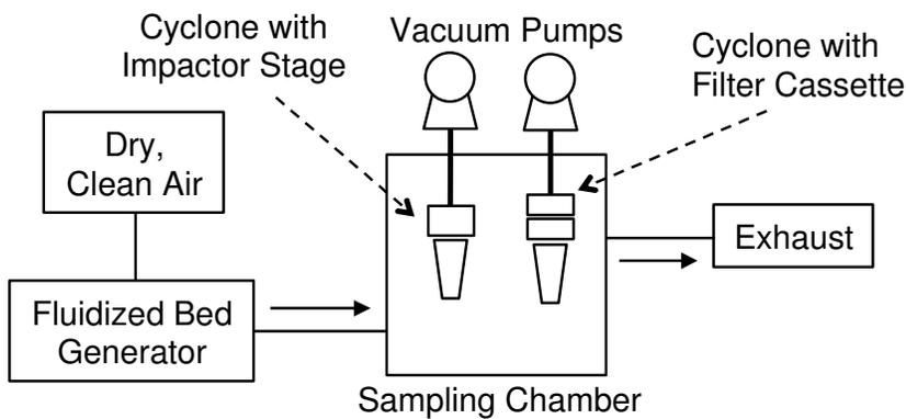
Figure S2. Experimental setup for the loading tests to evaluate the impactor's performance.
