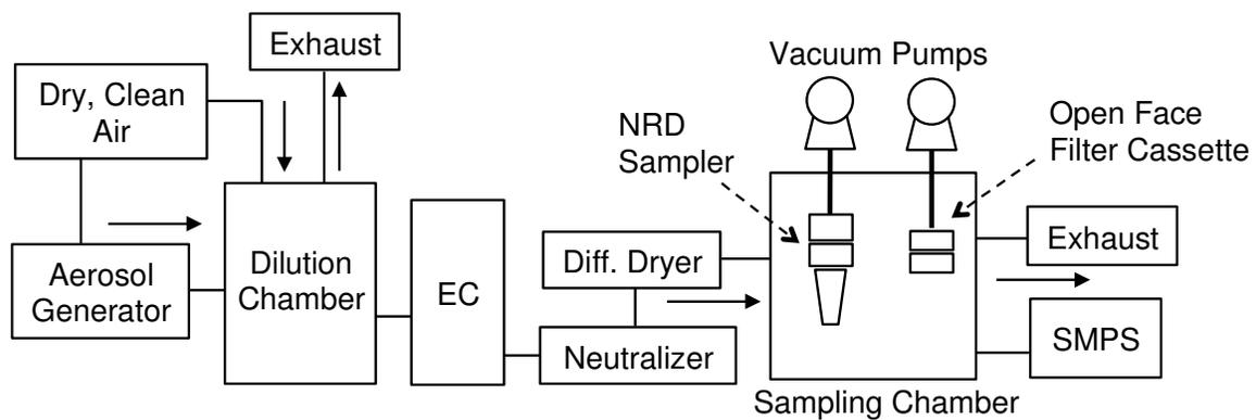
Figure S3. Experimental setup for the diffusion stage effective deposition tests.
