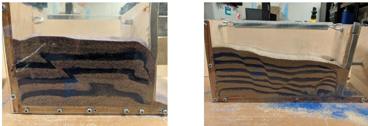
Figure 140: Examples of deformation patterns of “sand box” experiments in which alternating layers of differently-colored sand undergo deformation. Pictures courtesy of the lab of Dennis Harry at Colorado State University.
