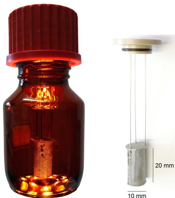
**Figure S2.** Drug release system designed in-house. The gel is loaded in the basket and the basket immersed in the release medium. A hole at the center of the beige cap (hole not seen on figure) makes sampling possible using a syringe fitted with a needle.
