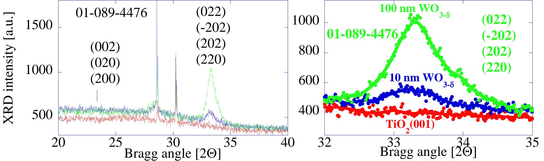
**Figure S1:** Comparison of X-ray diffractograms of clean  $\text{TiO}_2$  substrate and 10 nm and 100 nm as-deposited films grown on the same (001) substrate. The film peaks at  $33.4^\circ$  are identified with (022) of  $\text{WO}_3$ , see JCPDF reference card 01-089-4476.
