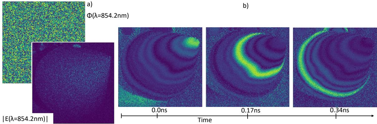
Fig. 2: Real world experiment (see Fig. 1c for setup description). a) Phase and amplitude of one single, captured optical (speckle) field ( $\lambda = 854.2nm$ ). b) Synthetic pulse computed from  $N = 21$  single optical speckle fields. The calculated intensity of the synthetic field is shown at three different time instances ( $0ns$ ,  $0.17ns$ ,  $0.34ns$ ), while the synthetic pulse is advancing through the scene. Full video can be found [here](#)
