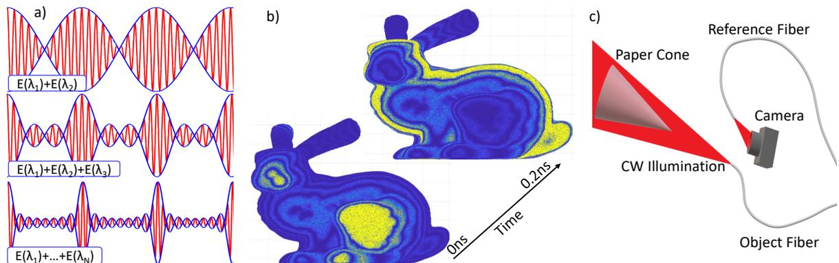
Fig. 1: a) Schematic: Real parts of synthetic fields created by addition of multiple optical fields  $E(\lambda_n)$ . b) Simulation: Synthetic pulse traveling across a 3D model c) Schematic of our experimental setup: A CW tunable laser illuminates a paper cone. The camera captures different optical fields  $E(\lambda_n)$  via single-shot interferometry [6].
