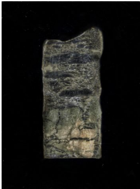
(Fig. 8) Contact images of permafrost core samples from the Yukon Research Centre
