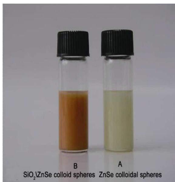
**Figure S3.** Photograph of ZnSe SPs and  $\text{SiO}_2@\text{ZnSe}$  SPs.
