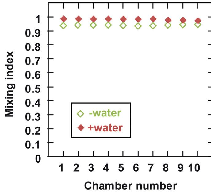
**Figure S4.** Evolution of the mixing index calculated as shown in figure 2C with or without the water phase.  $Q_{oil} = 0.5 \mu\text{L min}^{-1}$ ;  $Q_{water} = 5 \mu\text{L min}^{-1}$ ; acquisition time: 10 ms.
