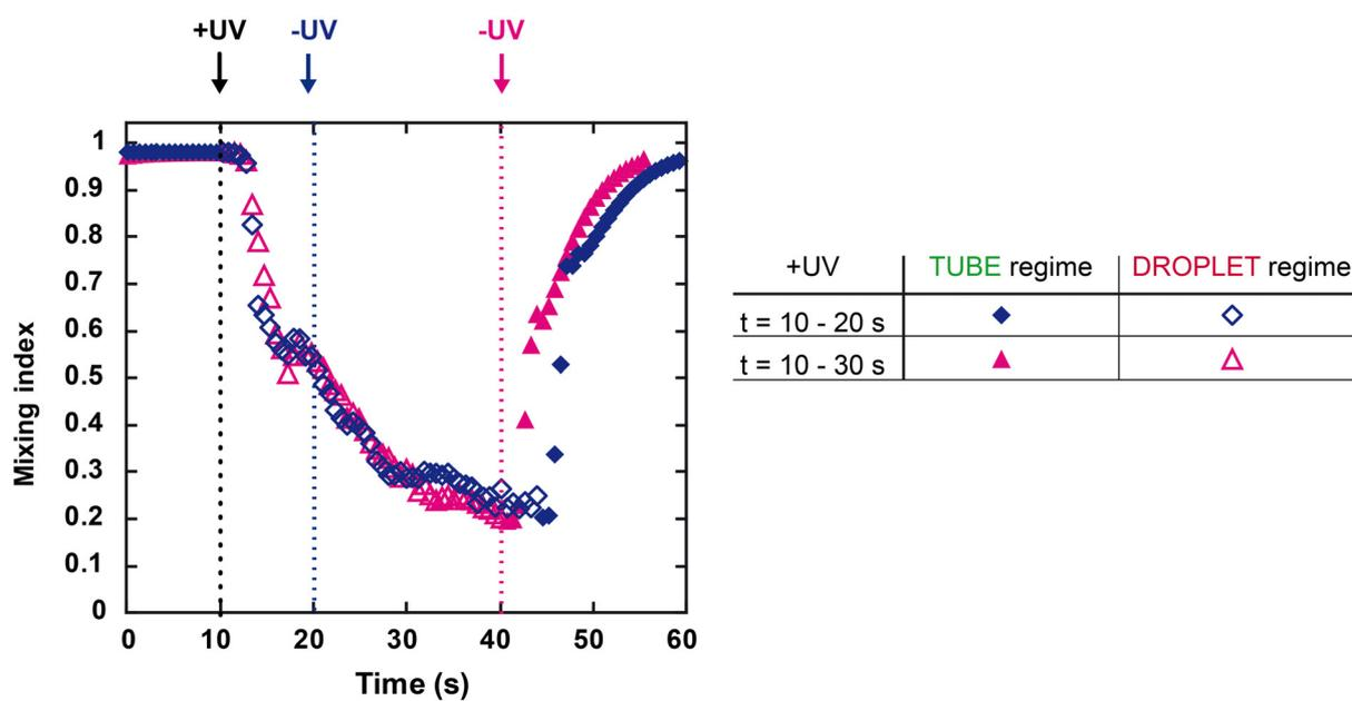
**Figure S7. Mixing index as a function of time for two experiments.** UV is applied at 10 s for all experiments (+UV, black dashed line) and removed at 20 s (blue diamonds) and 40 s (pink triangles)  $Q_{oil} = 0.5 \mu\text{L min}^{-1}$ ,  $Q_{water} = 2.5 \mu\text{L min}^{-1}$ ; acquisition time: 10 ms.
