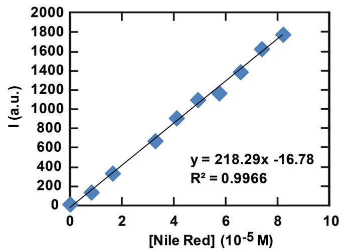
**Figure S2.** Correlation between the fluorescence intensity measured with fluorescent microscopy in the device and the concentration of Nile Red in oleic acid. Symbols are data points and the solid line is a linear fit.
