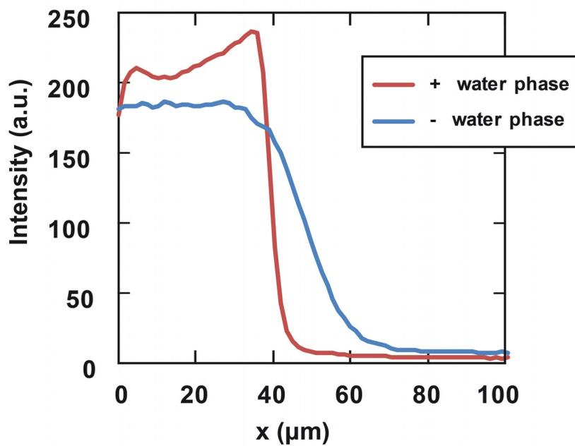
**Figure S3.** Intensity profile between the yellow arrow heads (top to bottom) for expansion chamber 10 in presence (red curve) and in absence (blue curve) of the water phase.  $Q_{oil} = 0.5 \mu\text{L min}^{-1}$ ;  $Q_{water} = 6 \mu\text{L min}^{-1}$ ; acquisition time: 10 ms.
