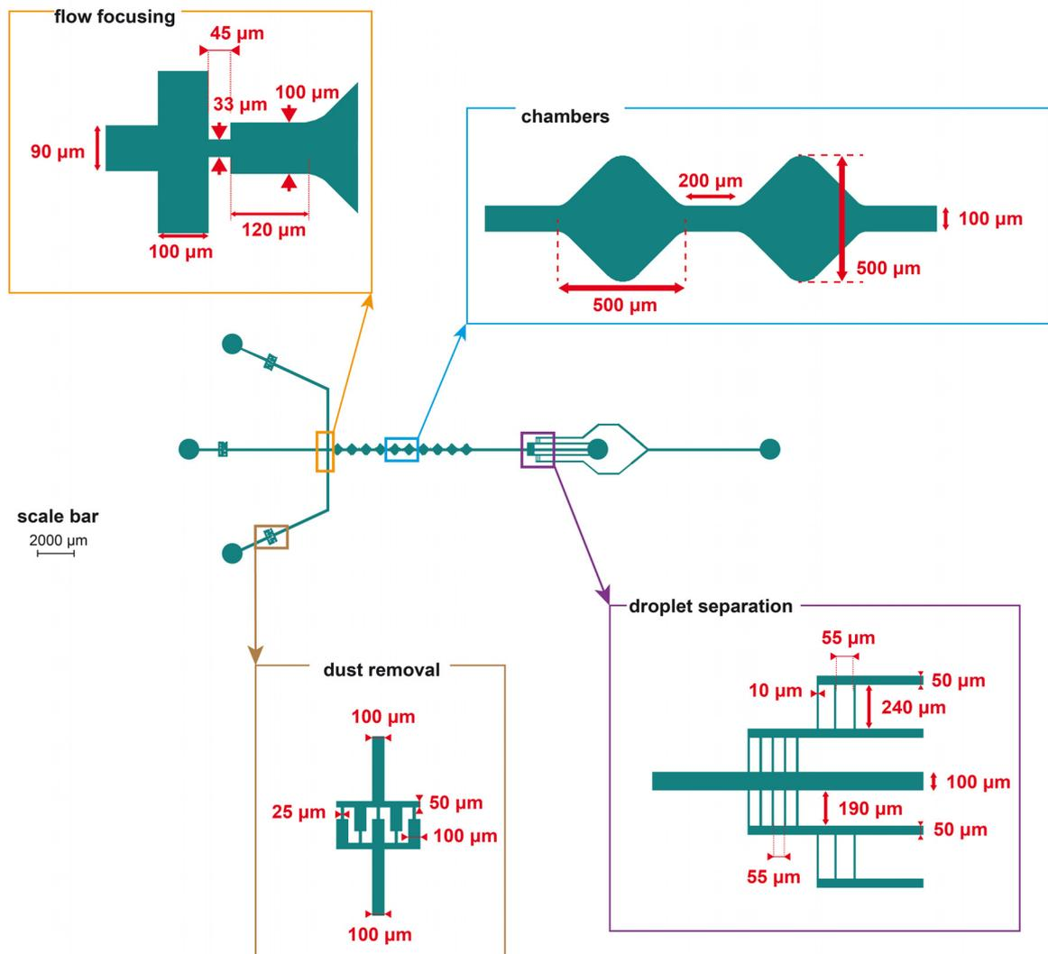
**Figure S1.** Full design is drawn to scale and the geometric characteristics of noteworthy regions are given.
