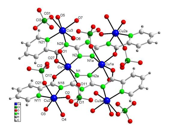
**S9.** Drawing of  $\mathbf{1}$  showing the (weak) interaction of the perchlorate anion Cl1 with Cu1.
