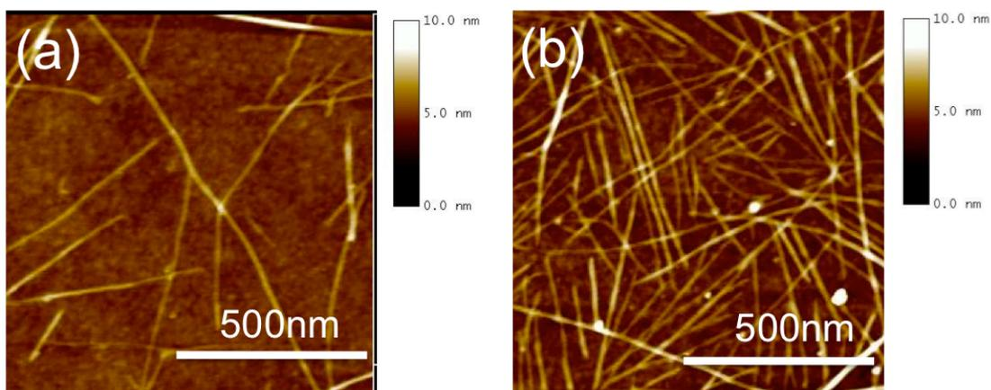
**Figure S4.** AFM images of the device made from large-diameter SWNTs with a density of (a)  $\sim 15$  SWNTs/ $\mu\text{m}^2$  (b)  $\sim 50$  SWNTs/ $\mu\text{m}^2$  dispersed by pDTFF-3T in toluene.
