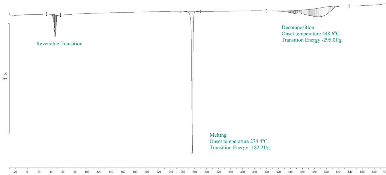
**Figure S 44.** Calorigram of lithium heptanoate determined by DSC over the range of  $T/^{\circ}\text{C} = (-30 \text{ to } 600)$  at a heating rate of  $\beta/^{\circ}\text{C}\cdot\text{s}^{-1}$  (0.167) and  $1.7 \text{ mL}\cdot\text{s}^{-1}$  nitrogen flow.
