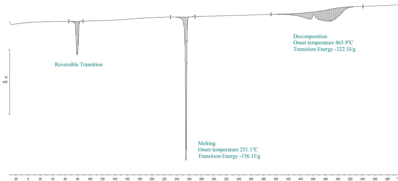
**Figure S 46.** Calorigram of lithium nonanoate determined by DSC over the range of  $T/^{\circ}\text{C} = (-30 \text{ to } 600)$  at a heating rate of  $\beta/^{\circ}\text{C}\cdot\text{s}^{-1}$  (0.167) and  $1.7 \text{ mL}\cdot\text{s}^{-1}$  nitrogen flow.
