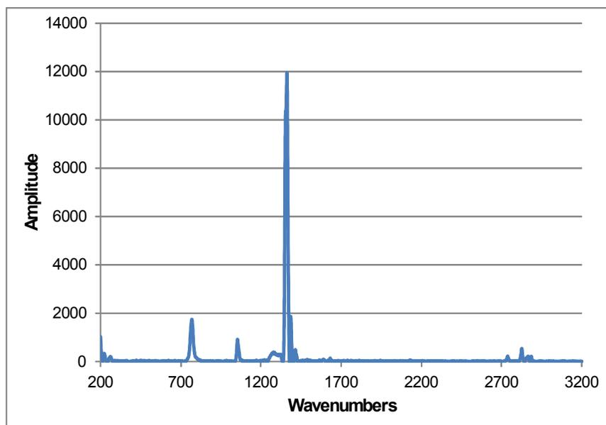
Figure S 13. Raman spectrum of lithium methanoate.
