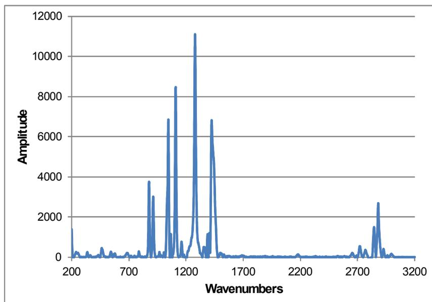
Figure S 23. Raman spectrum of lithium undecanoate.
