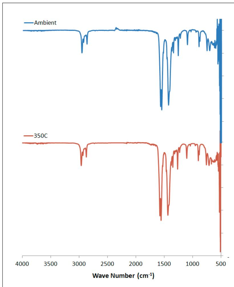
**Figure S 4.** IR spectrum of lithium butanoate before and after melting.
