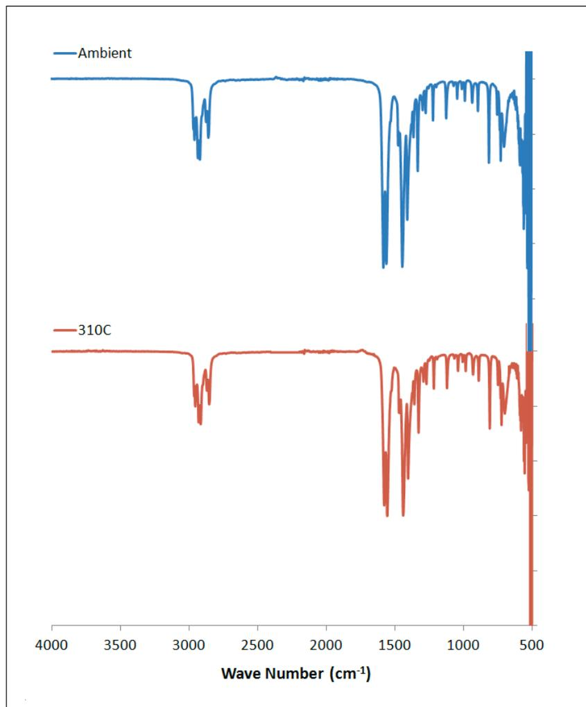
**Figure S 7.** IR spectrum of lithium heptanoate before and after melting.
