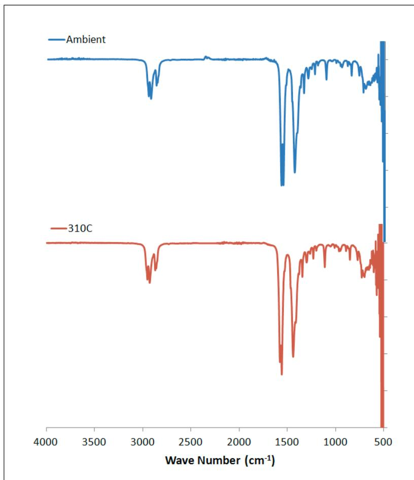
**Figure S 6.** IR spectrum of lithium hexanoate before and after melting.
