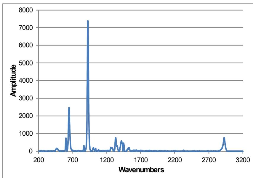
Figure S 14. Raman spectrum of lithium ethanoate.
