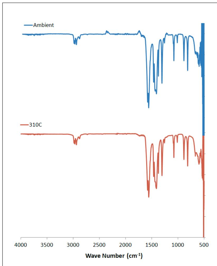
**Figure S 3.** IR spectrum of lithium propanoate before and after melting.
