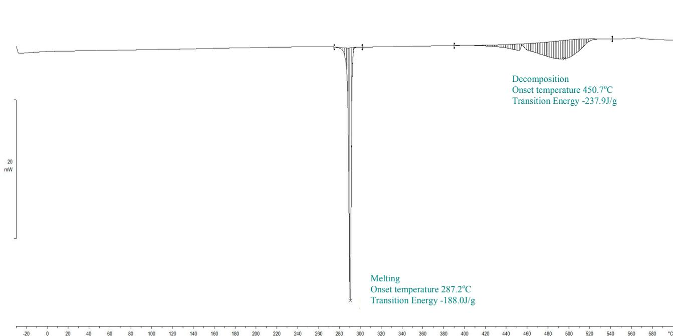
**Figure S 43.** Calorigram of lithium hexanoate determined by DSC over the range of  $T/^{\circ}\text{C} = (-30 \text{ to } 600)$  at a heating rate of  $\beta/^{\circ}\text{C}\cdot\text{s}^{-1}$  (0.167) and  $1.7 \text{ mL}\cdot\text{s}^{-1}$  nitrogen flow.
