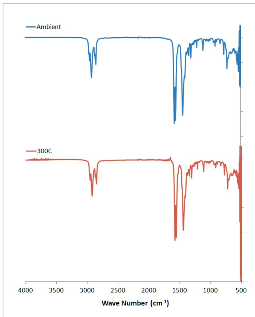
**Figure S 8.** IR spectrum of lithium octanoate before and after melting.
