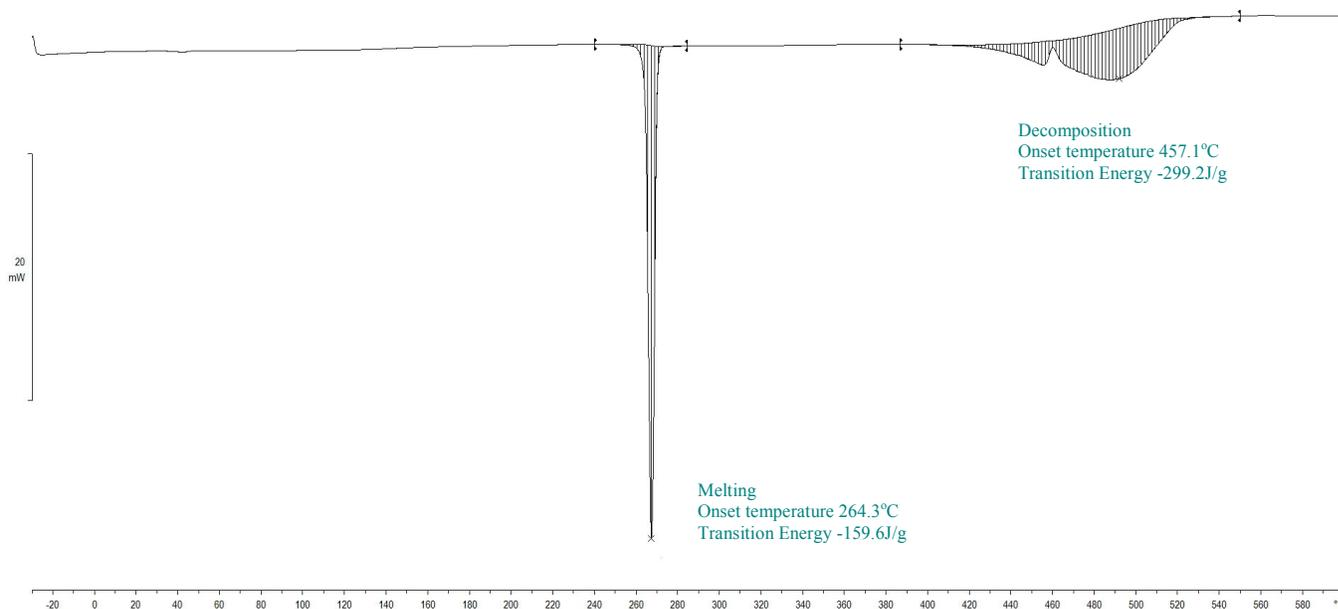
**Figure S 45.** Calorigram of lithium octanoate determined by DSC over the range of  $T/^{\circ}\text{C} = (-30 \text{ to } 600)$  at a heating rate of  $\beta/^{\circ}\text{C}\cdot\text{s}^{-1}$  (0.167) and  $1.7 \text{ mL}\cdot\text{s}^{-1}$  nitrogen flow.
