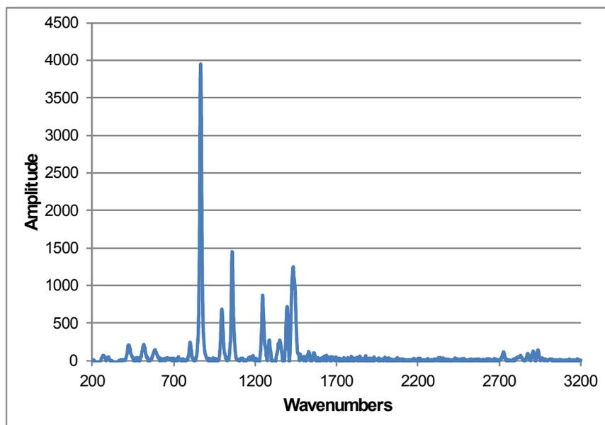
Figure S 15. Raman spectrum of lithium propanoate.
