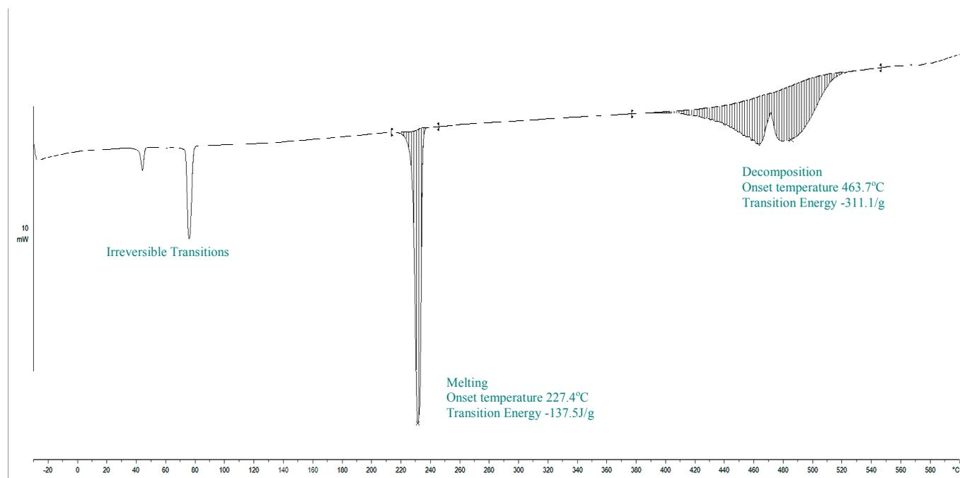
**Figure S 49.** Calorigram of lithium dodecanoate determined by DSC over the range of  $T/^\circ\text{C} = (-30 \text{ to } 600)$  at a heating rate of  $\beta/^\circ\text{C}\cdot\text{s}^{-1}$  (0.167) and  $1.7 \text{ mL}\cdot\text{s}^{-1}$  nitrogen flow.
