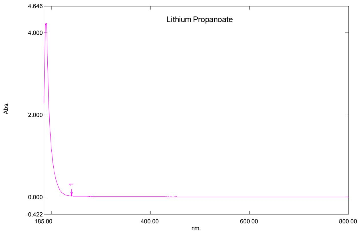
Figure S 27. UV-Vis spectrum of lithium propanoate.
