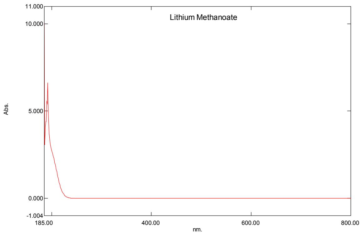
Figure S 25. UV-Vis spectrum of lithium methanoate.
