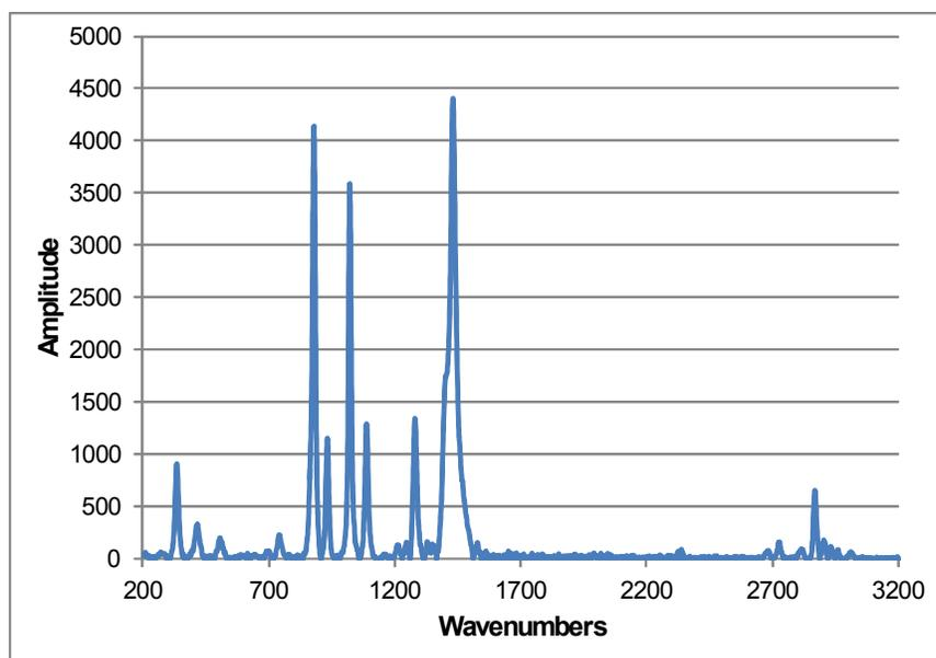
Figure S 16. Raman spectrum of lithium butanoate.
