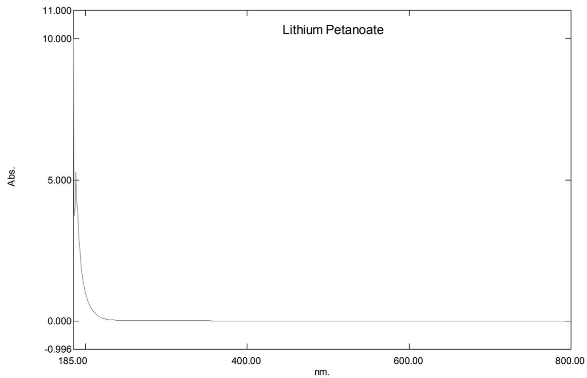
Figure S 29. UV-Vis spectrum of lithium pentanoate.
