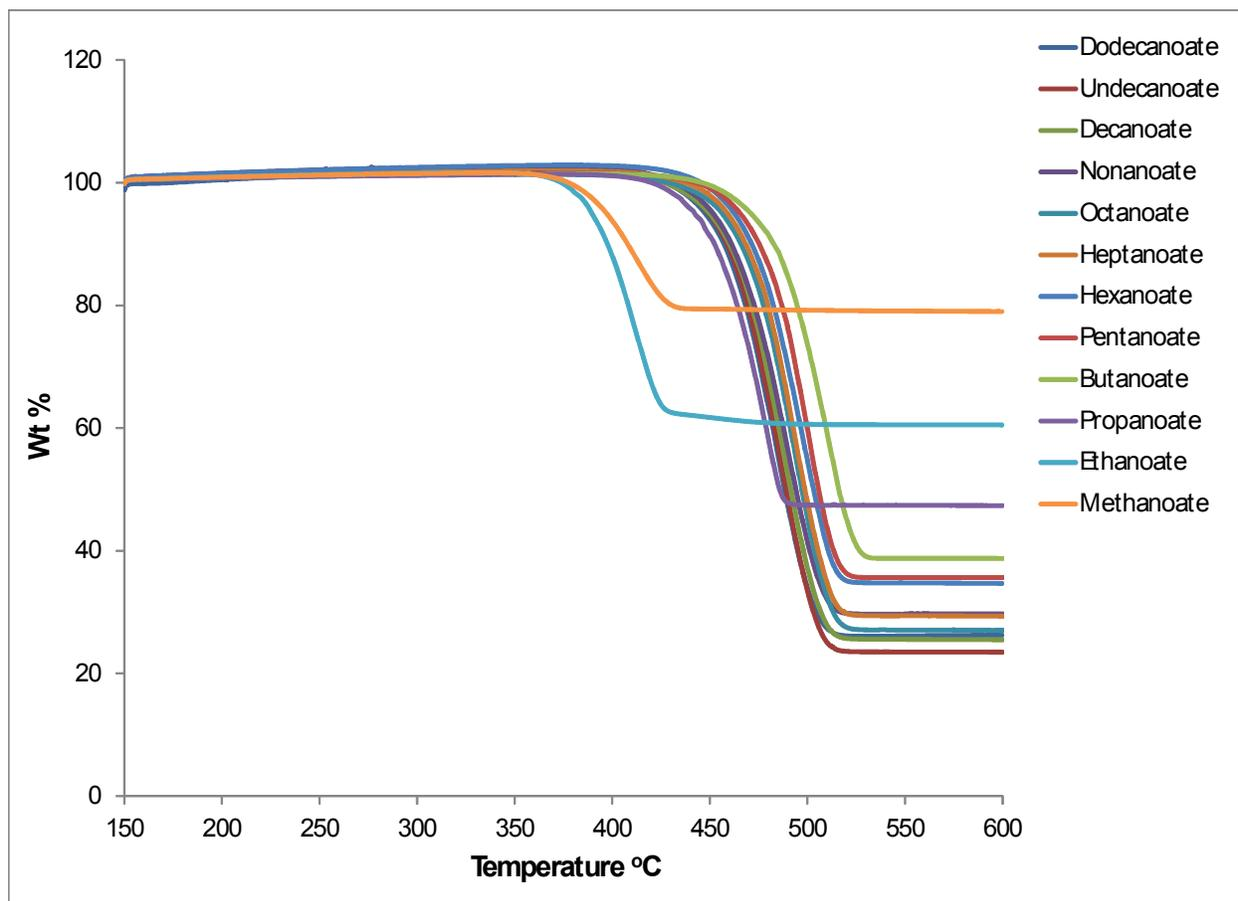
**Figure S 37.** TGA mass loss with temperature of the  $C_1$ - $C_{12}$  Li-carboxylates over the range  $T/^\circ\text{C} = (150 \text{ to } 600)$  at a heating rate of  $\beta/^\circ\text{C}\cdot\text{s}^{-1}$  (0.167) and conducted under inert atmosphere ( $\text{N}_2$ ).
