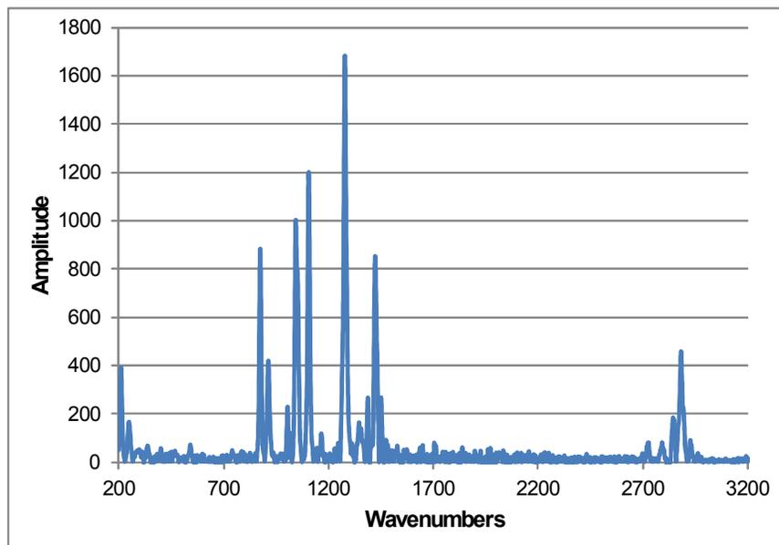
Figure S 21. Raman spectrum of lithium nonanoate.
