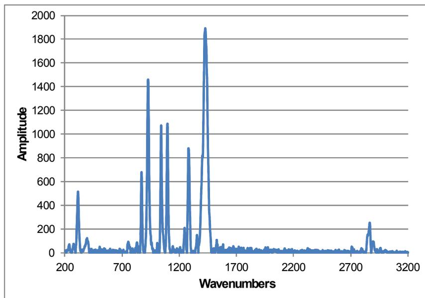
Figure S 18. Raman spectrum of lithium hexanoate.
