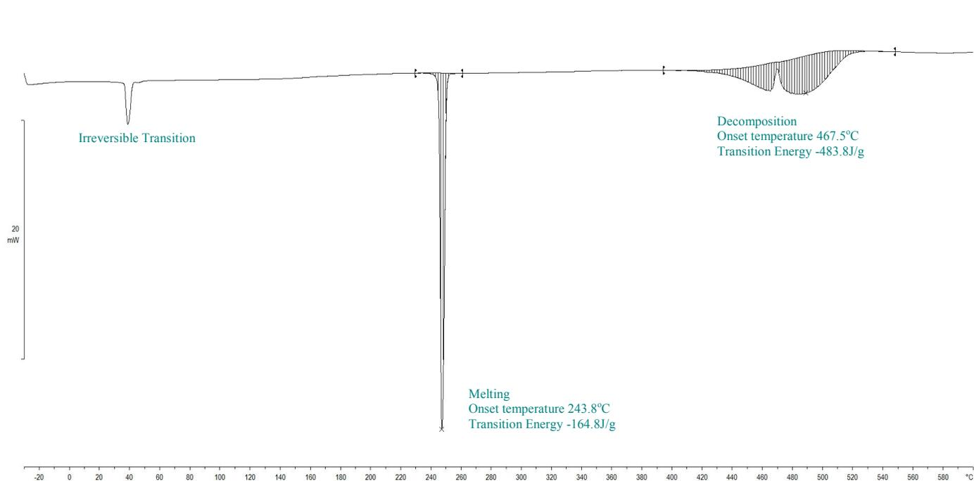
**Figure S 47.** Calorigram of lithium decanoate determined by DSC over the range of  $T/^{\circ}\text{C} = (-30 \text{ to } 600)$  at a heating rate of  $\beta/^{\circ}\text{C}\cdot\text{s}^{-1}$  (0.167) and  $1.7 \text{ mL}\cdot\text{s}^{-1}$  nitrogen flow.
