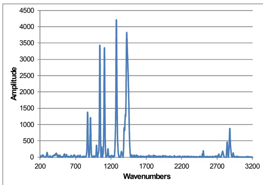
Figure S 24. Raman spectra of lithium dodecanoate.
