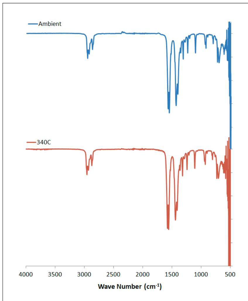
**Figure S 5.** IR spectrum of lithium pentanoate before and after melting.
