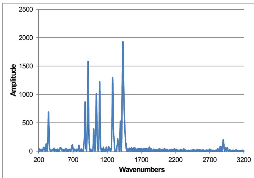
Figure S 17. Raman spectrum of lithium pentanoate.
