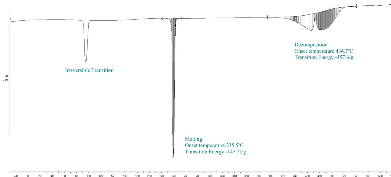
**Figure S 48.** Calorigram of lithium undecanoate determined by DSC over the range of  $T/^{\circ}\text{C} = (-30 \text{ to } 600)$  at a heating rate of  $\beta/^{\circ}\text{C}\cdot\text{s}^{-1}$  (0.167) and  $1.7 \text{ mL}\cdot\text{s}^{-1}$  nitrogen flow.
