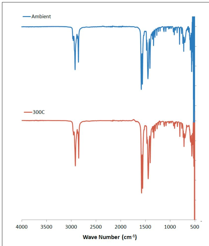
**Figure S 11.** IR spectrum of lithium undecanoate before and after melting.
