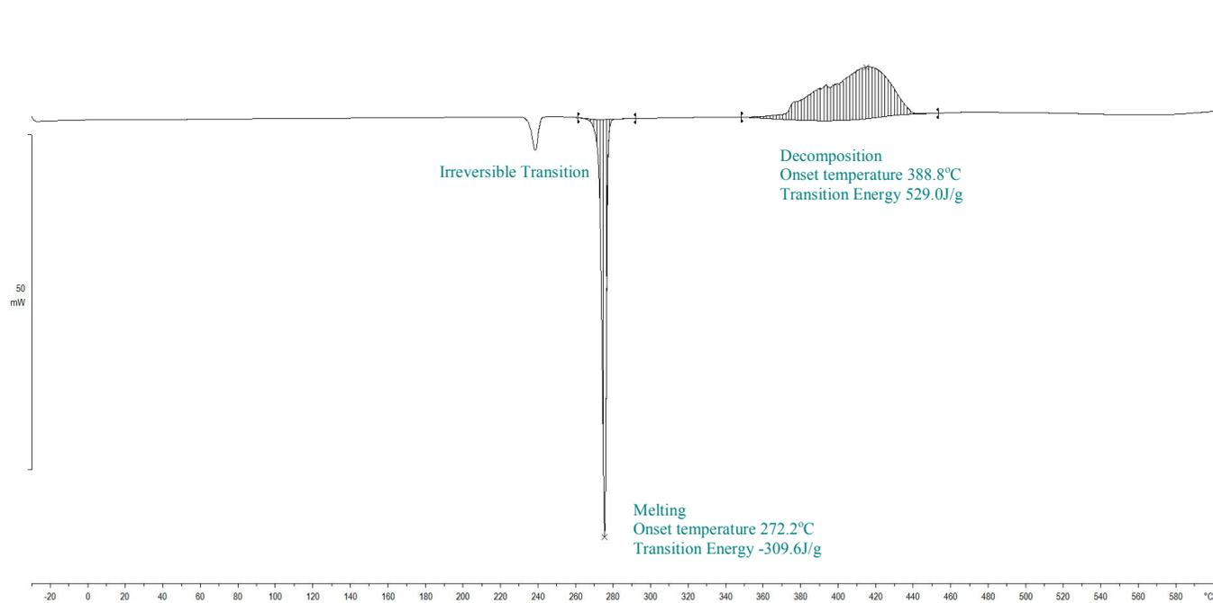
**Figure S 38.** Calorigram of lithium methanoate determined by DSC over the range of  $T/^\circ\text{C} = (-30 \text{ to } 600)$  at a heating rate of  $\beta/^\circ\text{C}\cdot\text{s}^{-1}$  (0.167) and  $1.7 \text{ mL}\cdot\text{s}^{-1}$  nitrogen flow.
