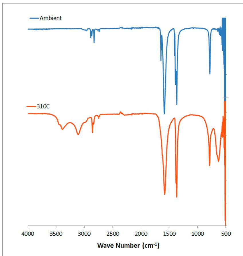
**Figure S 1.** IR spectrum of lithium methanoate before and after melting.
