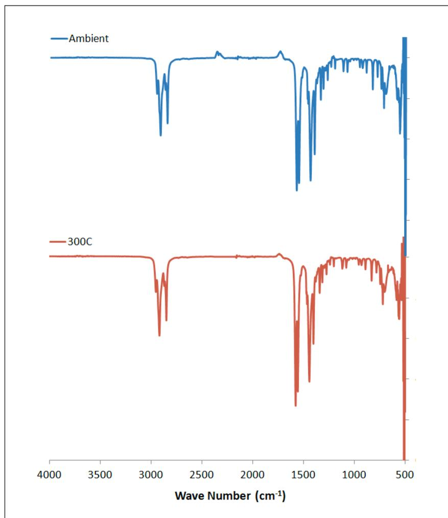
Figure S 10. IR spectrum of lithium decanoate before and after melting.
