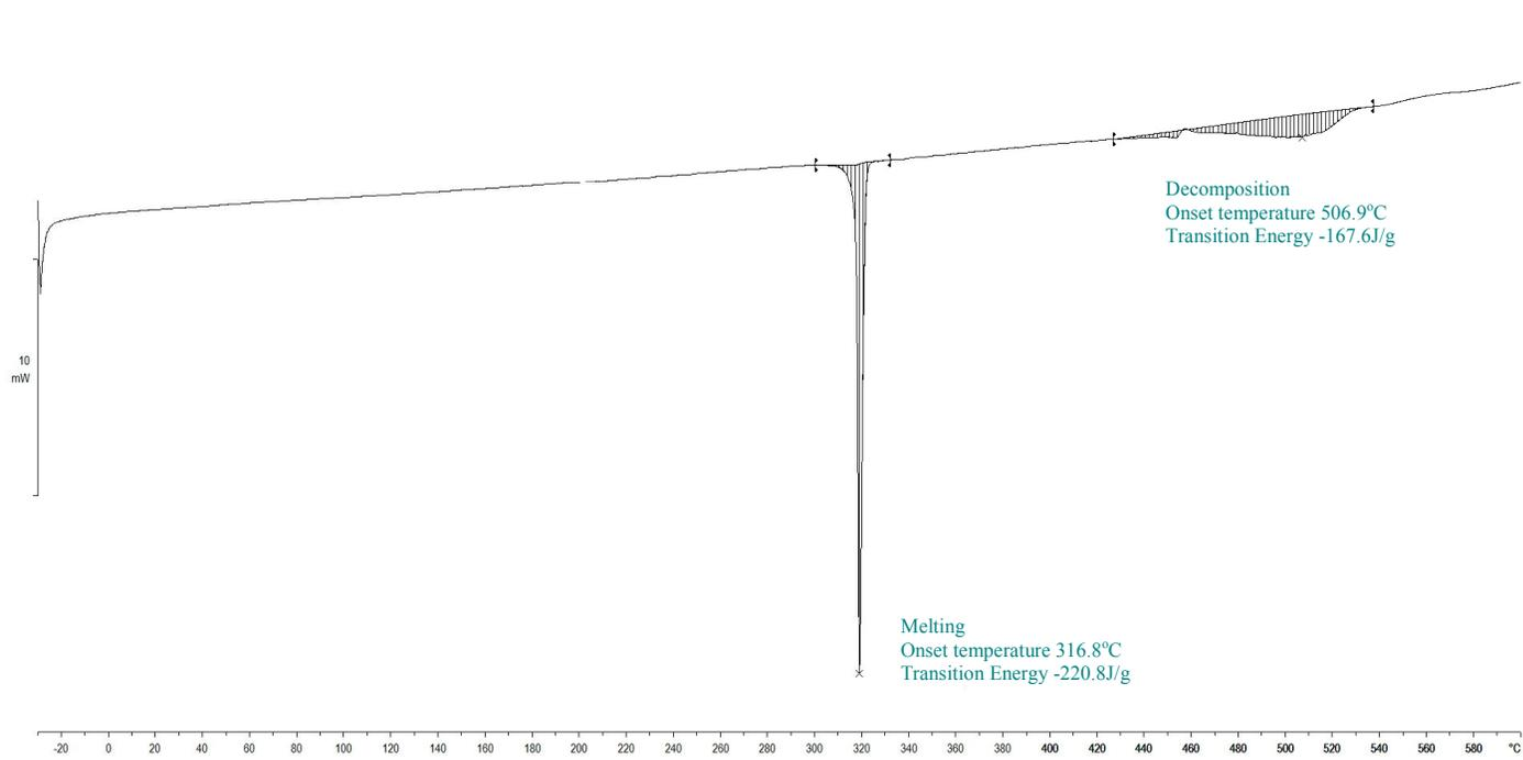
**Figure S 41.** Calorigram of lithium butanoate determined by DSC over the range of  $T/^{\circ}\text{C} = (-30 \text{ to } 600)$  at a heating rate of  $\beta/^{\circ}\text{C}\cdot\text{s}^{-1}$  (0.167) and  $1.7 \text{ mL}\cdot\text{s}^{-1}$  nitrogen flow.
