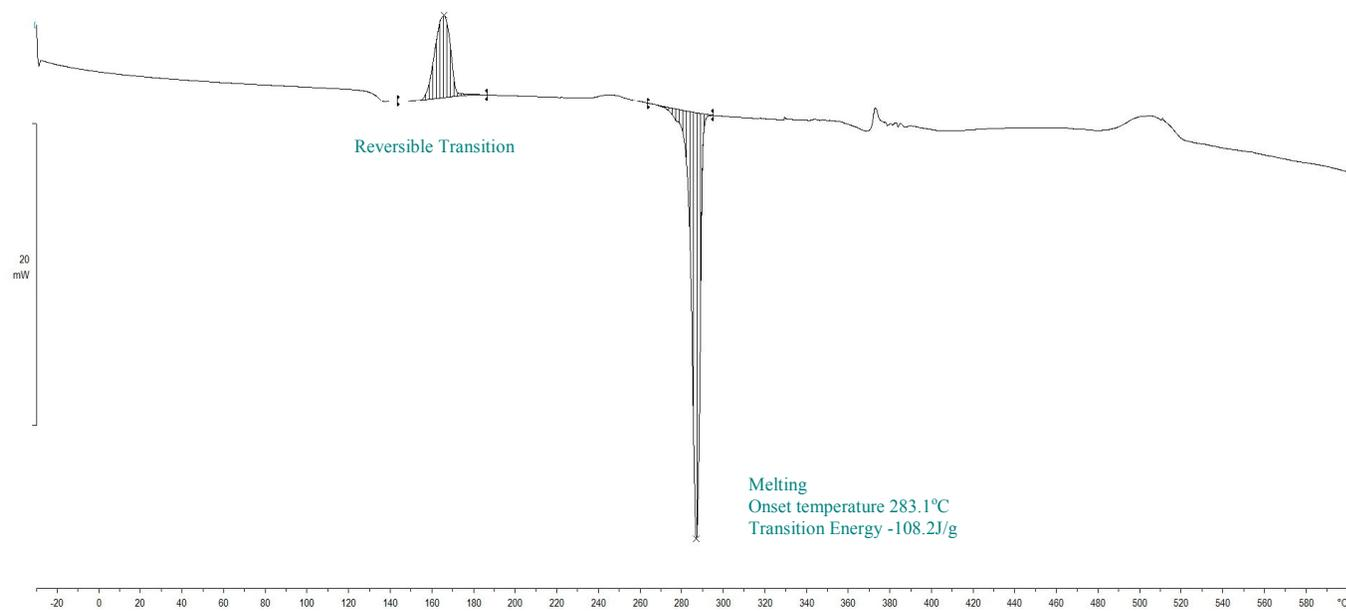
**Figure S 39.** Calorigram of lithium ethanoate determined by DSC over the range of  $T/^{\circ}\text{C} = (-30 \text{ to } 600)$  at a heating rate of  $\beta/^{\circ}\text{C}\cdot\text{s}^{-1}$  (0.167) and  $1.7 \text{ mL}\cdot\text{s}^{-1}$  nitrogen flow.
