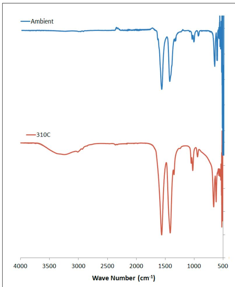
**Figure S 2.** IR spectrum of lithium ethanoate before and after melting.
