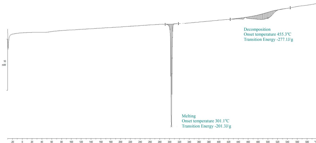
**Figure S 42.** Calorigram of lithium pentanoate determined by DSC over the range of  $T/^{\circ}\text{C} = (-30 \text{ to } 600)$  at a heating rate of  $\beta/^{\circ}\text{C}\cdot\text{s}^{-1}$  (0.167) and  $1.7 \text{ mL}\cdot\text{s}^{-1}$  nitrogen flow.
