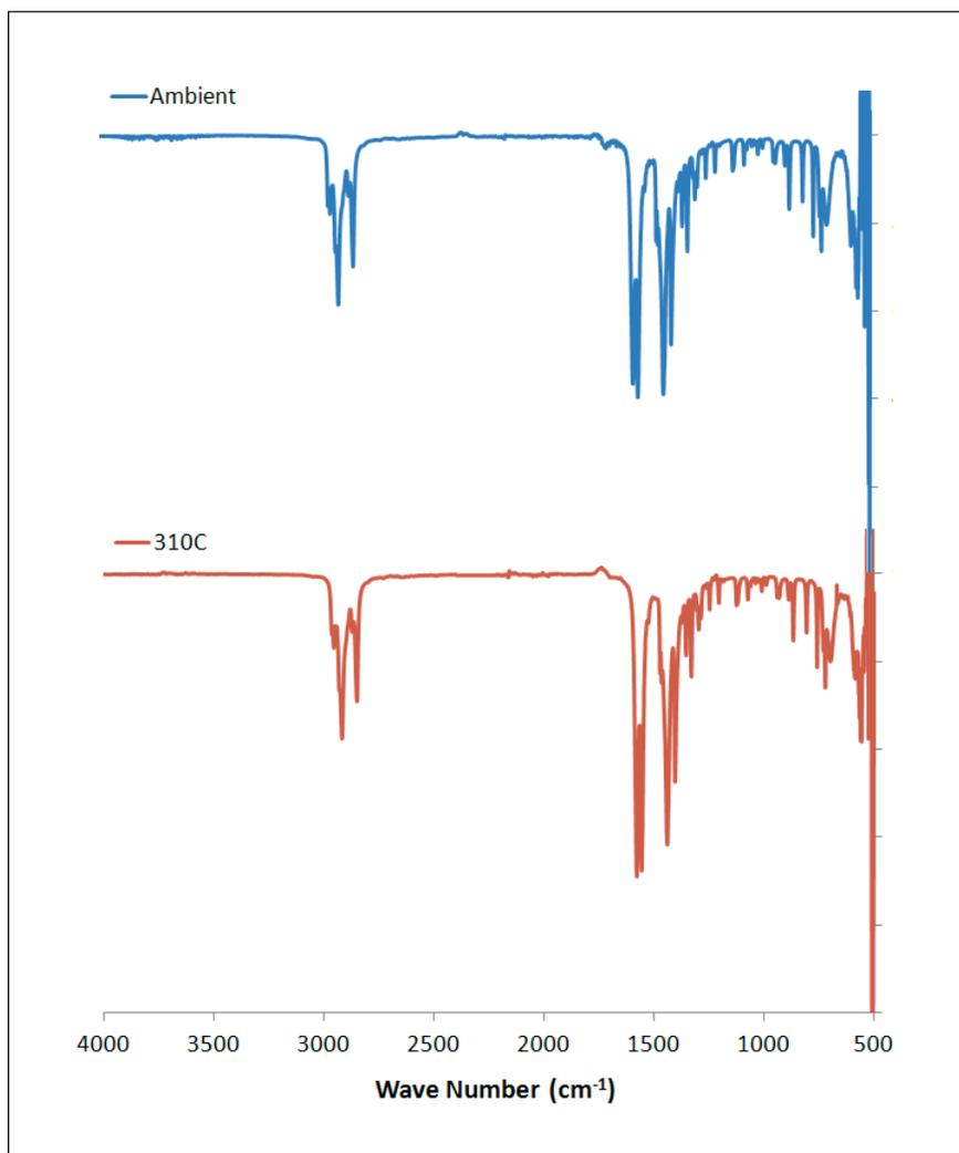
**Figure S 9.** IR spectrum of lithium nonanoate before and after melting.
