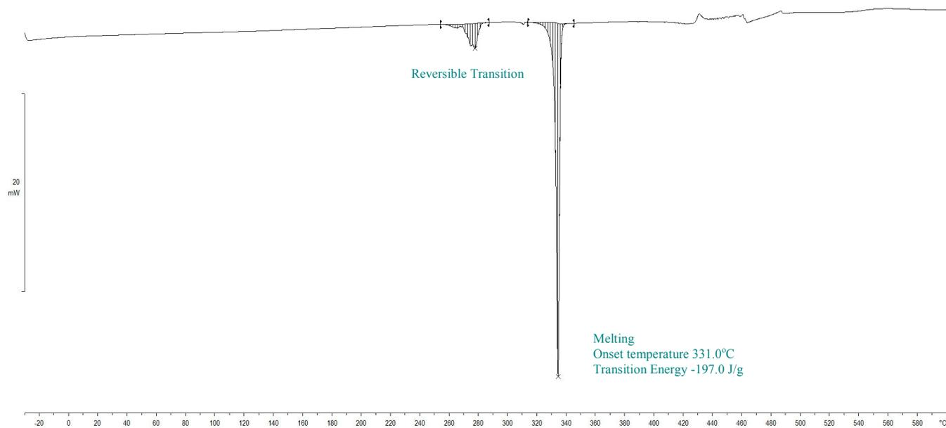
**Figure S 40.** Calorigram of lithium propanoate determined by DSC over the range of  $T/^{\circ}\text{C} = (-30 \text{ to } 600)$  at a heating rate of  $\beta/^{\circ}\text{C}\cdot\text{s}^{-1}$  (0.167) and  $1.7 \text{ mL}\cdot\text{s}^{-1}$  nitrogen flow.
