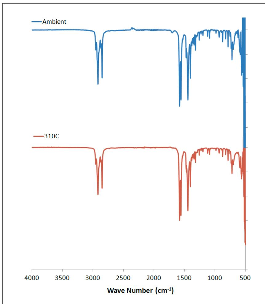
Figure S 12. IR spectrum of lithium dodecanoate before and after melting.
