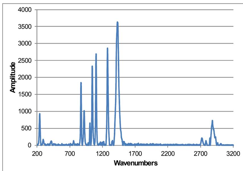
Figure S 20. Raman spectrum of lithium octanoate.
