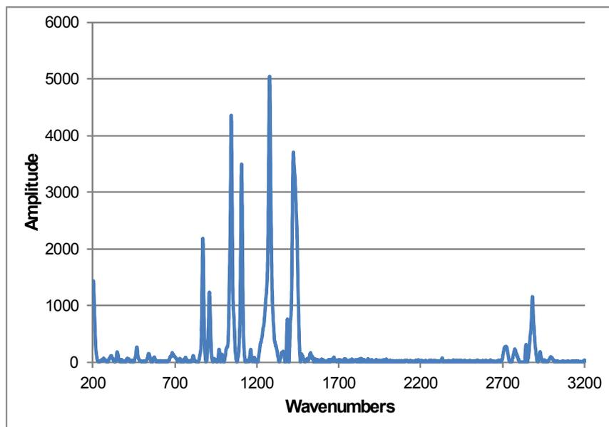
Figure S 22. Raman spectrum of lithium decanoate.
