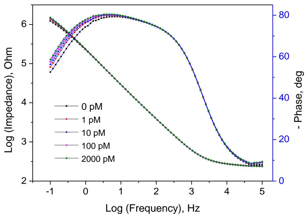
**Figure S2** Non-Faradaic EIS Bode plots of the biosensor interfaces after exposure to calibrated concentrations of insulin. Measurements in 10 mM PBS (pH 7.4) across a frequency range of 0.1-100K Hz. Note that, in the lower frequency range, phase change is substantially more significant than the impedance change.
