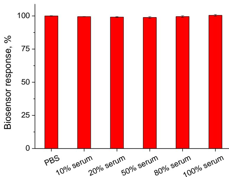
**Figure S4** Biosensor response to 50 pM insulin in progressively increasing serum concentration with the response in pure PBS taken as 100%. The response is based on the EIS phase change before and after insulin spiking, and the assay errors are within 2%. Error bars represent the standard deviations of three measurement repeats.
