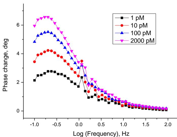
**Figure S3** Neat phase changes of the biosensor interfaces after exposure to different concentrations of insulin. Data recorded in PBS (10 mM, pH 7.4) with the highest response at 0.2 Hz [ $\log(0.2) = -0.7$ ]. The fluctuation in the middle of the curves is a potentiostat artefact that does not impact measurements.
