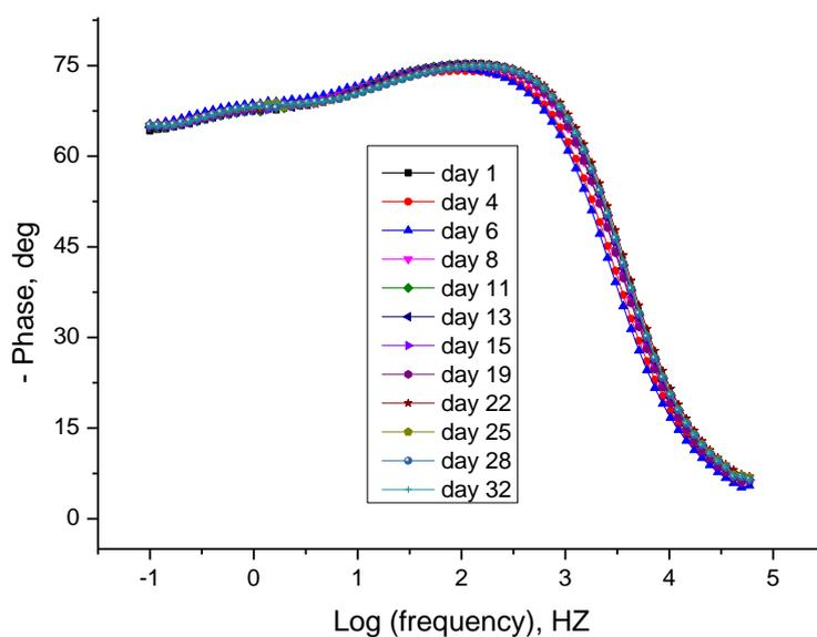
**Figure S1** Non-Faradaic EIS Bode phase plots of the electrode modified with PCBMA as recorded at different time intervals in PBS (10 mM, pH 7.4). The excellent interfacial stability is evident (the relative standard deviation of the recorded phase at 0.2 Hz is less than 0.5%).
